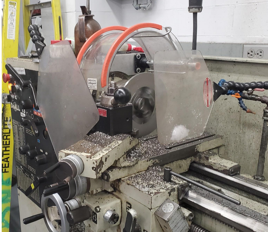
Figure 49: Brake Rotor on the Lathe
