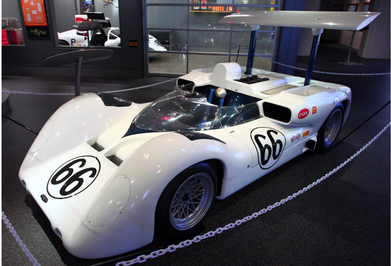
Figure 13: The 1966 Chaparral 2E, showing its rear wing
