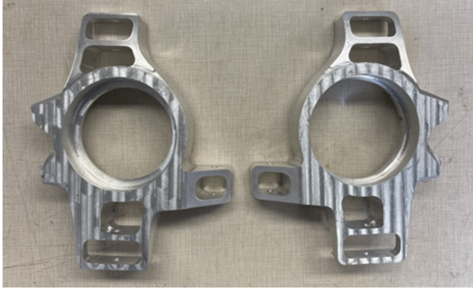
Figure 24: Finished rear uprights
