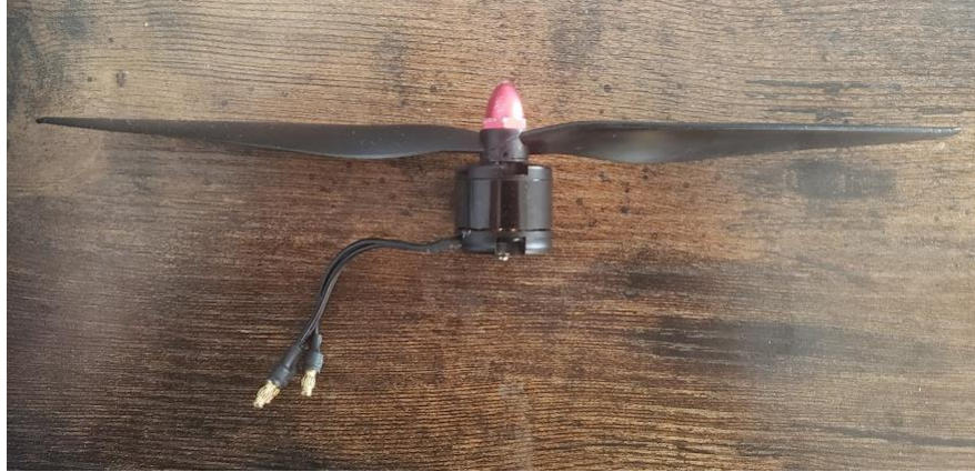
Fig. 3.7. Emax Mt2213 935kV Brushless Motor with 1045 Propeller.
