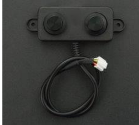
Fig. 3.13. A02YYUW Waterproof Ultrasonic sensor. [19]
