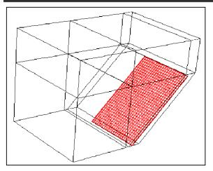
Figure 14 -- Isometric view of the no-slip wall boundary condition applied to the exterior surface of the 3-layer windshield that is exposed to fluid.
