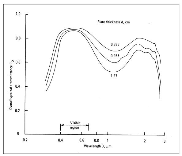
Figure 3 -- Spectral transmittance, including surface reflection, for soda-lime glass.
