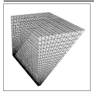
Figure 6 – "Above\_Eng" grid object that represents the airspace above the hood between the windshield and fire objects. The grid dimensions are 16x36x32.
