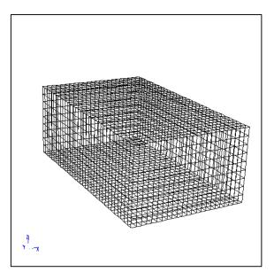
Figure 8 – "Above\_Fire" grid object representing the fluid region above the "Fire" object. The grid dimensions are 24x36x12.
