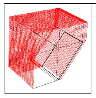
Figure 16 -- Isometric view of opening boundary condition applied to all exterior boundaries of the computational domain that are exposed to fluid.
