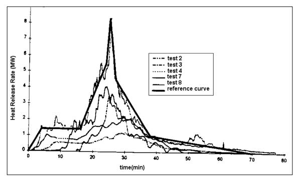
Figure 1-- ProfilARBED design heat release rate for a burning motor vehicle plotted with experimental heat release rates.
