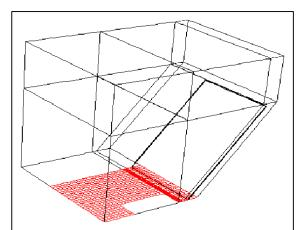
Figure 13 -- Isometric view of the no-slip wall boundary condition applied to the hood of the vehicle. This reveals the fluid extension beside the hood which is used to capture the flow field of air near the vehicle.
