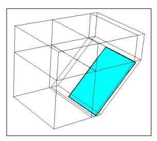
Figure 11 -- Isometric view of assembled TASCflow model for the windshield problem. The attachments between the six grid objects presented in this section can be seen.
