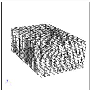
Figure 9 – "Top\_Front" grid object representing the fluid region above the "Above\_Eng" object. The grid dimensions are 16x36x12.
