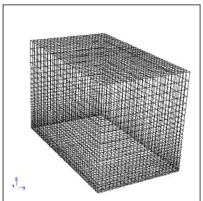
Figure 7 -- The "Fire" grid object which represents the airspace above the hood and contains the combustion region. The grid dimensions are 24x36x32.
