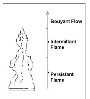
Figure 2 -- Burning regions of a typical turbulent diffusion flame.
