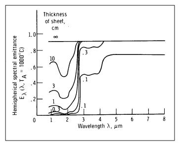
Figure 4 -- Spectral emission of soda-lime glass at 1000 C.
