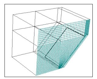
Figure 12 -- Isometric view of the symmetry boundary condition applied to the TASCflow windshield model.
