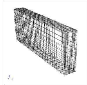
Figure 10—"Top\_Mid" grid object representing the fluid region above the windshield grid object. The grid dimensions are 15x36x12.
