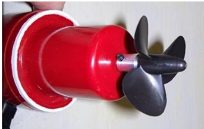
Figure 37: Modified Bilge Pump
