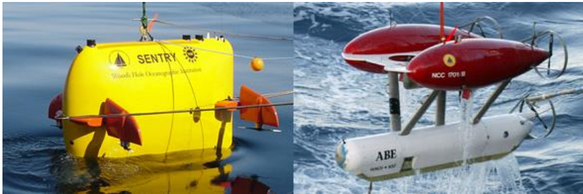
Figure 3: Non-Torpedo Shaped AUVs: SENTRY (left) [19] and ABE (right) [20]
