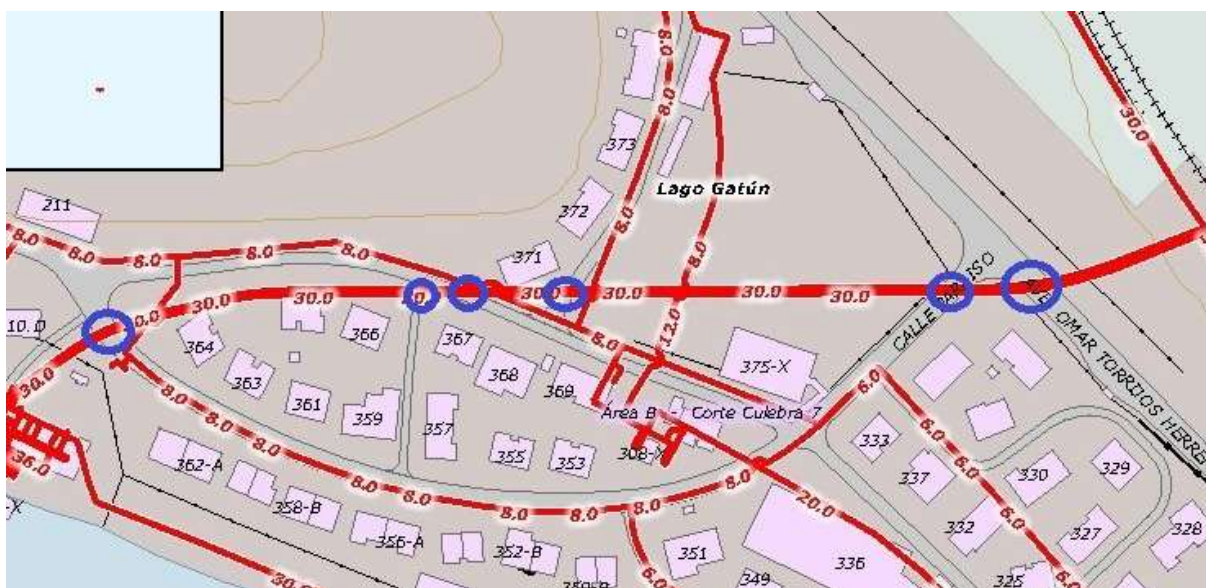
Figure 26 - North line leaving the Paraíso Pumping Station and approaching the Gamboa line (ACP Internal GIS System, 2012)
