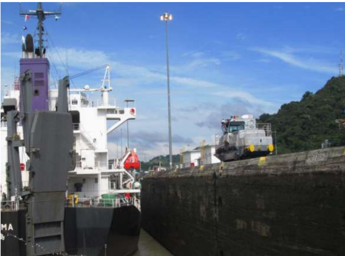
Figure 5 - Locomotive Guiding a Ship in the Pedro Miguel Locks (Photo Taken by Shelby Miller, 2012)
