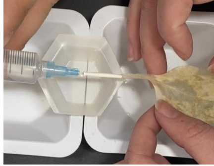
Figure 27: Flow Test with Micro Tubing and Electrospun material
