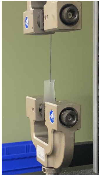
Figure 21: Suture retention testing setup using the Instron 5544
