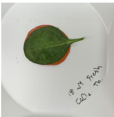
Figure 18: Spinach leaf attached to patch with 18mM calcium chloride solution in fibrin glue
