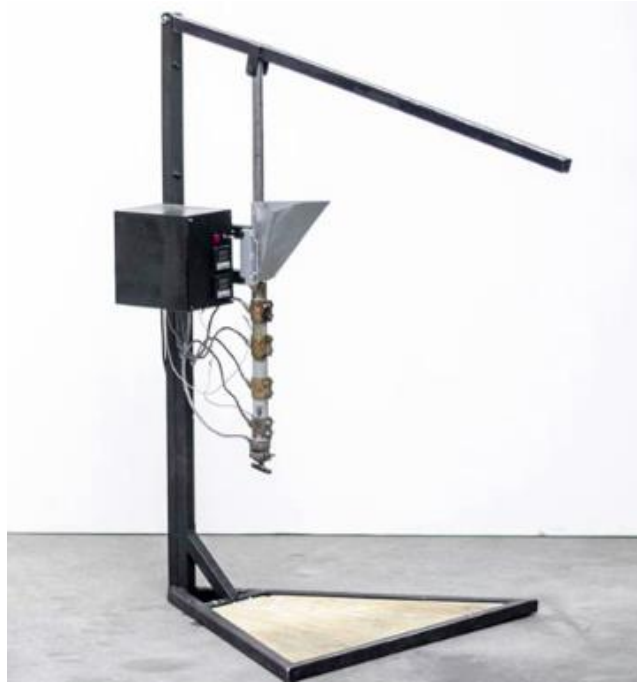
Figure 5: Injection Machine (Precious Plastic, 2020) " Injection " by Precious Plastic is licensed under CC BY 4.0
