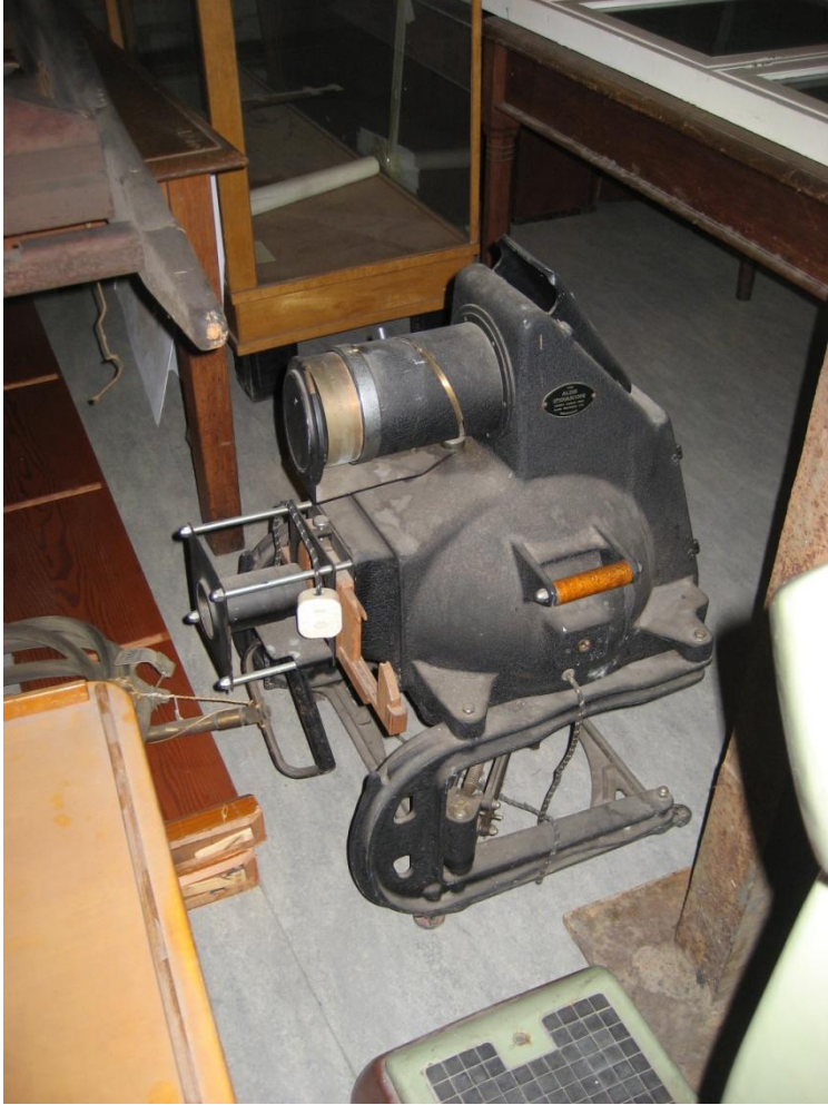
Figure b.1.9 An original limelight projector converted to electric power.
