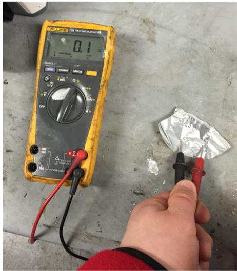
*Figure 42: Resistance testing of current collector materials*
