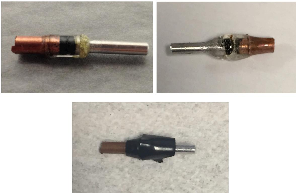
*Figure 33: Top Left: Fully assembled PGE separator battery. Top Right: Fully assembled gap separator battery. Bottom: Micro-battery with electrical tape wrapping for light shielding*
