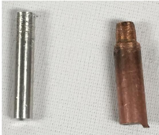
*Figure 22: Aluminum dowel pin current collector after sanding to insure interference fit (Left) Copper current collector after machining and sanding (Right)*
