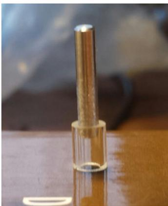
*Figure 27: Aluminum dowel pin current collector prior to sealing. Dowel pin and glass cylinder form a interference fit.*
