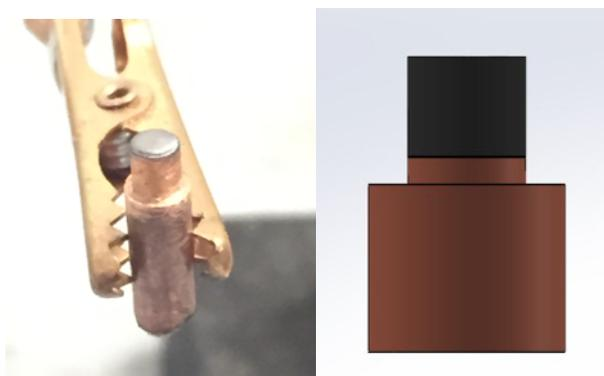
Figure 32: Post processing images of anode deposition onto copper current collect. Actual process (Left) Schematic of process (Right)
