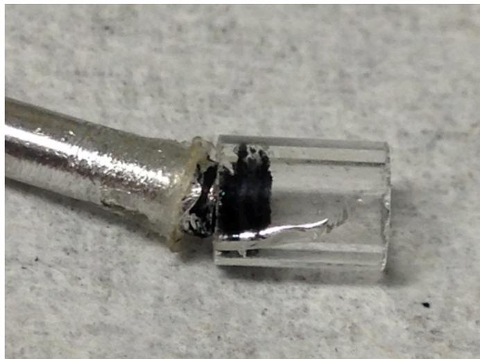
*Figure 53: Example of a battery housing breaking during processing*
