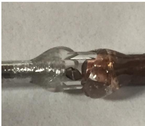
*Figure 23: Lithium metal sealed inside battery prior to hermiticity test*
