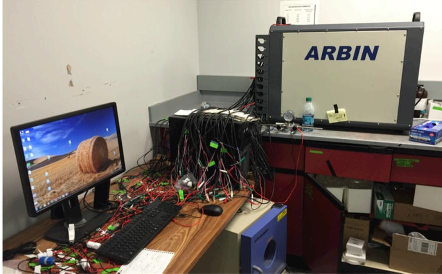
Figure 34: The ARBIN electrochemical testing system with testing module and computer shown
