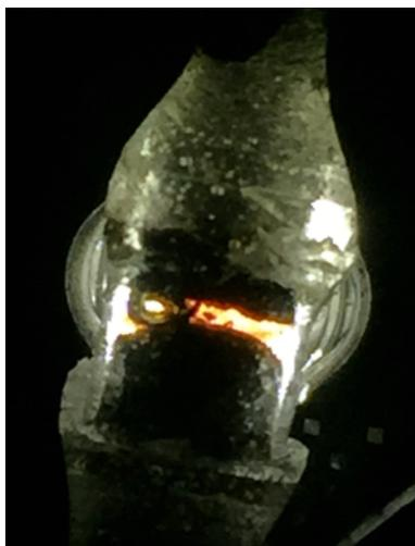
*Figure 30: LED backlit image of gap separator battery*
