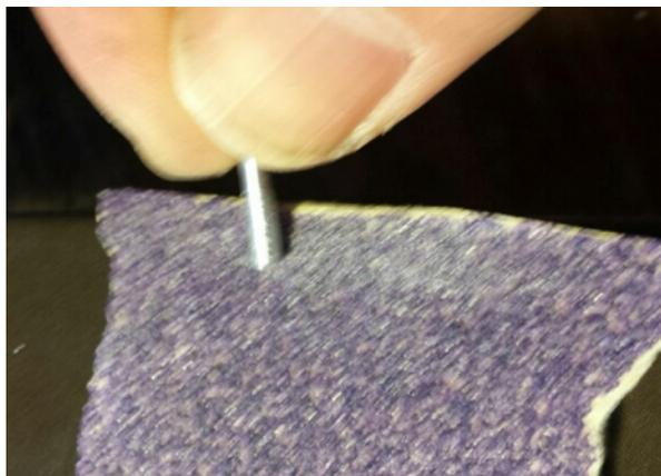
*Figure 21: Aluminum current collector being sanded*
