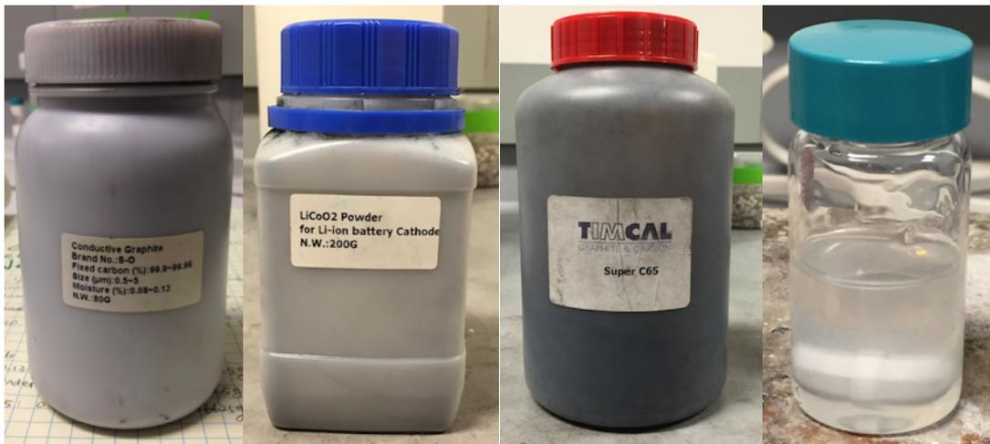
Figure 25: Electrode components from left to right: Conductive Graphite, LiCoO<sub>2</sub> Powder, C65 Carbon, 2.5% Binder Solution of PVDF in NMP
