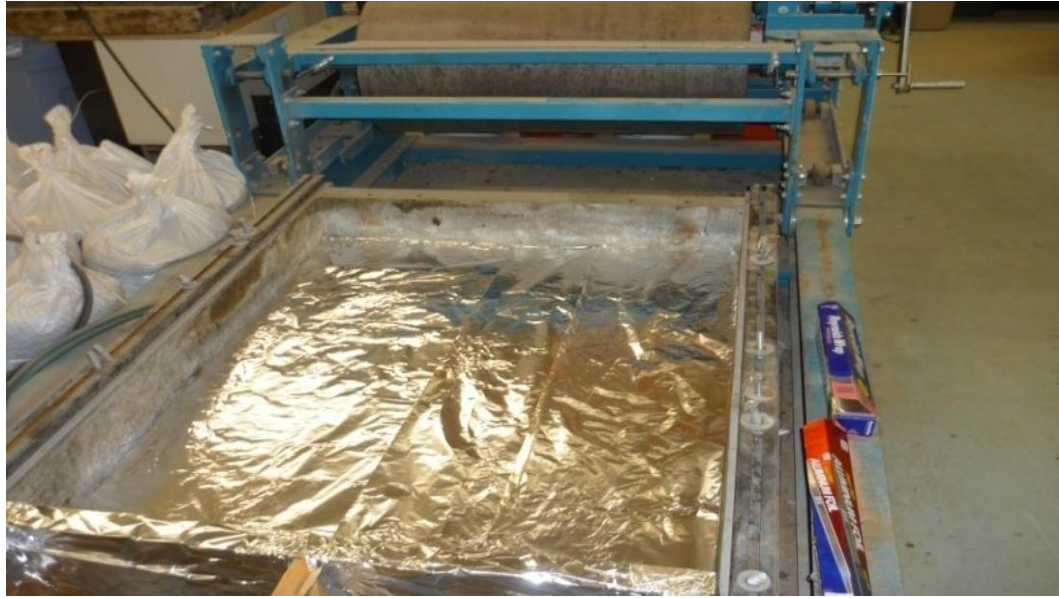
Figure 17 : Foil sheet covered the wood board
