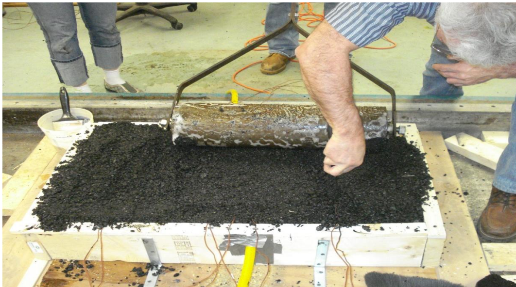
Figure 25: Compaction of Extra 0.35 in Layer
