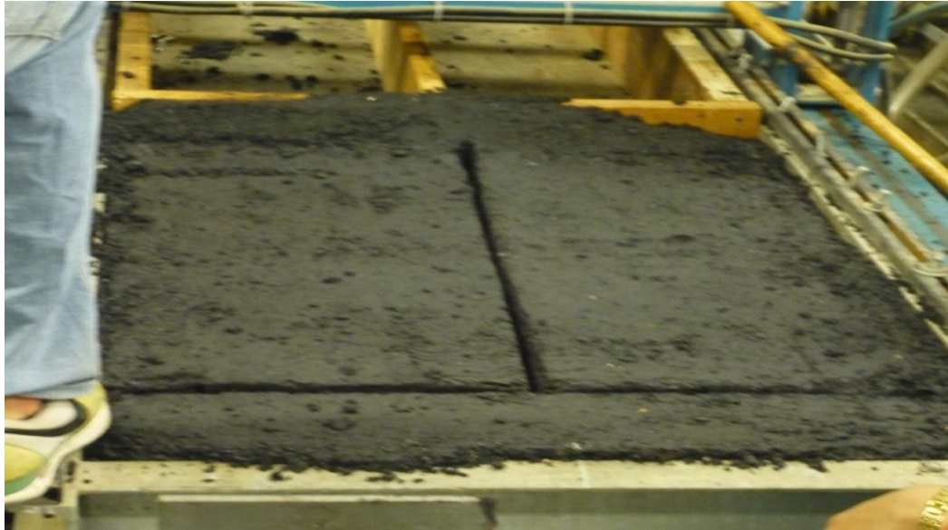
Figure 20: Cutting the Slab Longitudinally Into Two Halves
