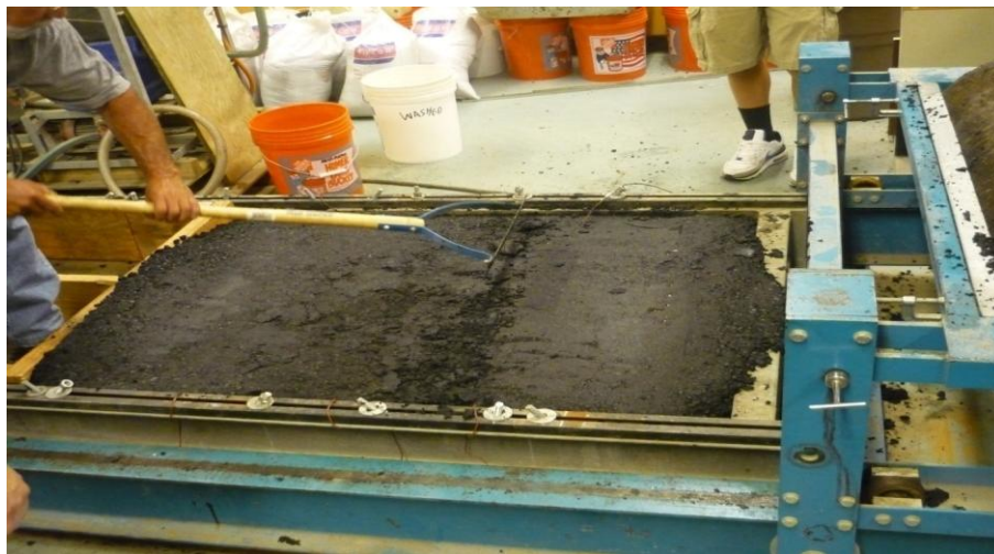
Figure 23: Compaction of Hot Mix Asphalt in the Slab
