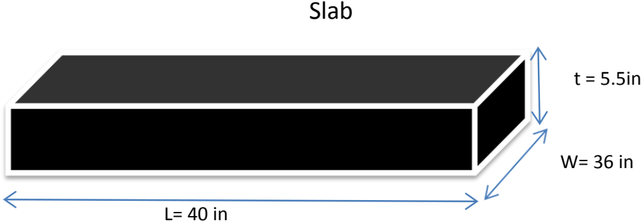
Figure 19: Present the Slab Dimensions
