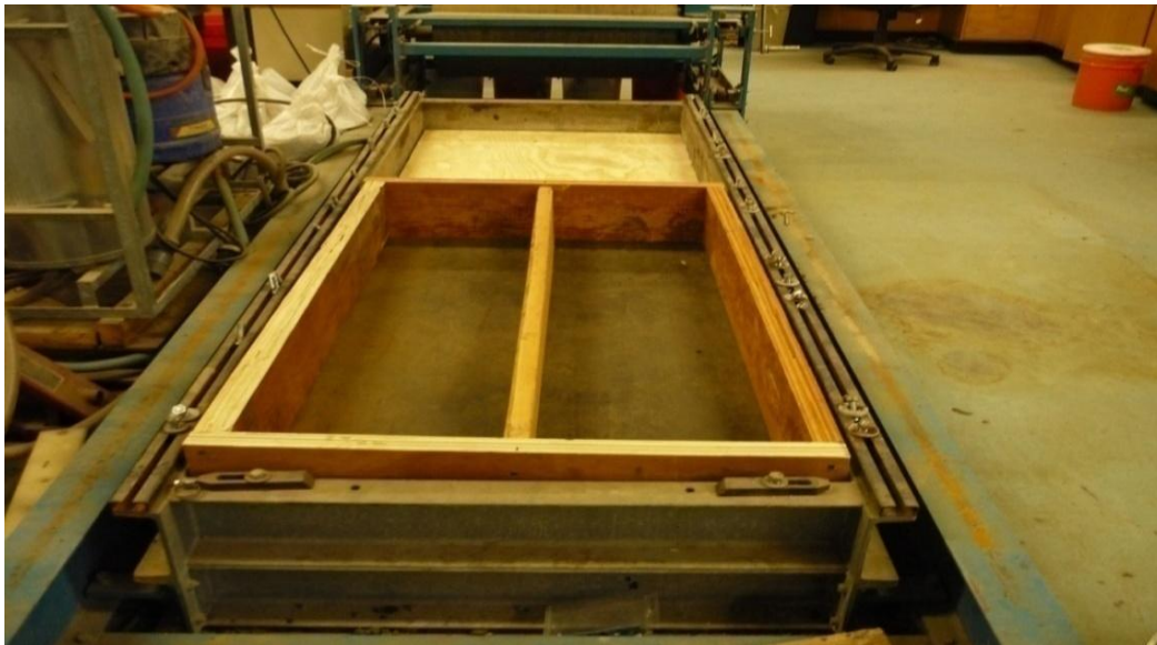
Figure 18 : Wood Frame Support Slab's End
