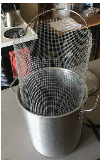
Figure 4. Second iteration of the wire mesh strainer in the kettle
