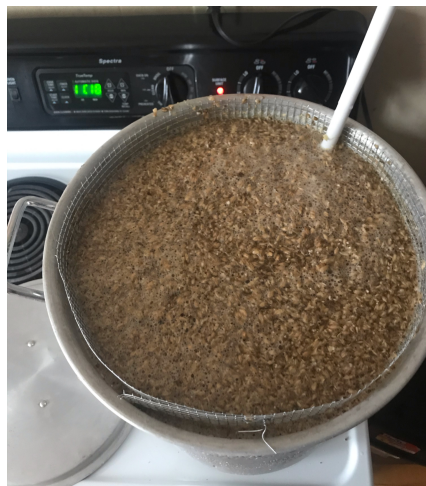
Figure 7. Second iteration of the wire mesh strainer during the brewing process
