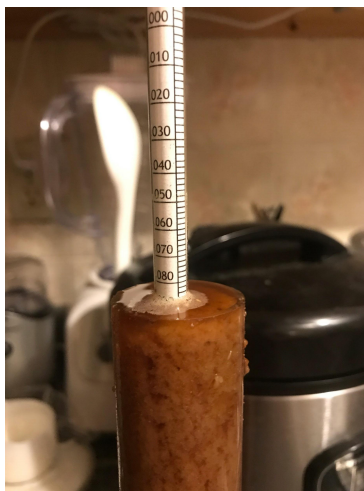
Figure 5. Specific Gravity Reading of 1.086 for Batch #9
