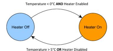
Figure 43: Operation of the Heater [58] © 2016 Clyde Space Ltd.
