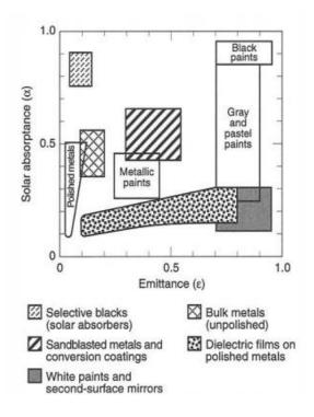
**Figure 14:** Surface Absorptivity and Emissivity of Various Types of Materials [41] Copyright © 2017 The Aerospace Press
