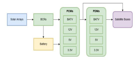
Figure 25: EPS Board Power Flow
