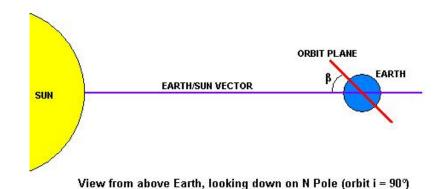
**Figure 95:** Beta Angle of Satellite [70]. Copyright © 2005 Colorado Center for Astrodynamics Research.
