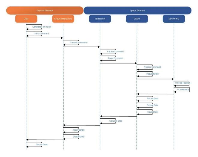
Figure 52: Request Payload Data Diagram
