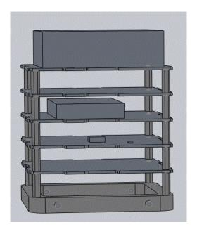
Figure 39: Simplified Circuit Stack with Heat Dissipating Components
