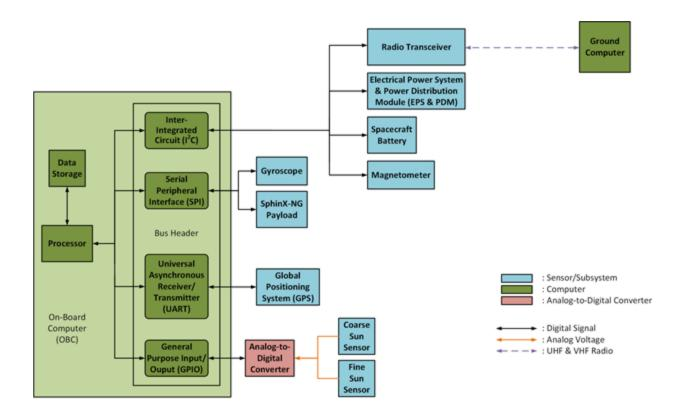
Figure 55: Command and Data Handling Subsystem Block Diagram
