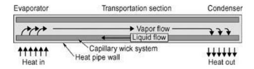
Figure 16: Schematic of Heat Pipe System [42] Copyright © 2002 AIAA
