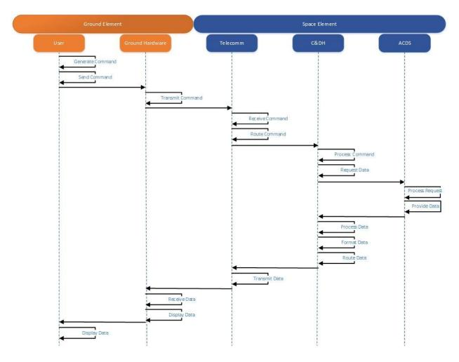
Figure 53: Request Telemetry Diagram
