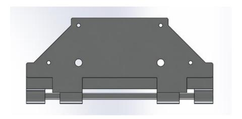
Figure 34: 2013 MQP CubeSat Solar Panel Hinge [1] Copyright © 2013 WPI
