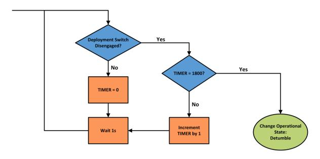
Figure 47: P-POD Deployment Operational State
