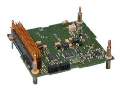
Figure 11: ISIS UHF/VHF Transceiver [32] Copyright © 2017 CubeSatShop.com
