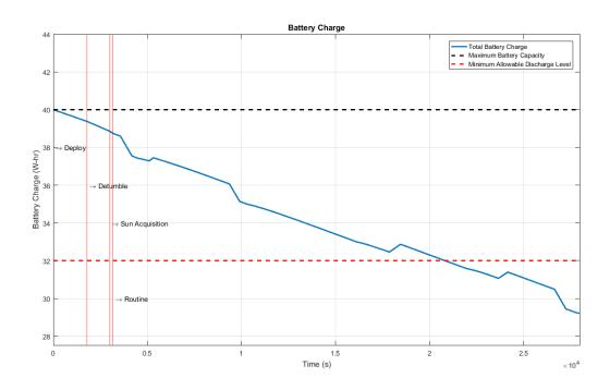
Figure 71: Battery Charge vs. Time
