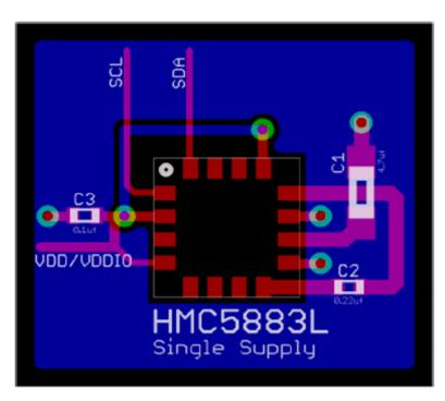
Magnetometer Application Circuit [81]
