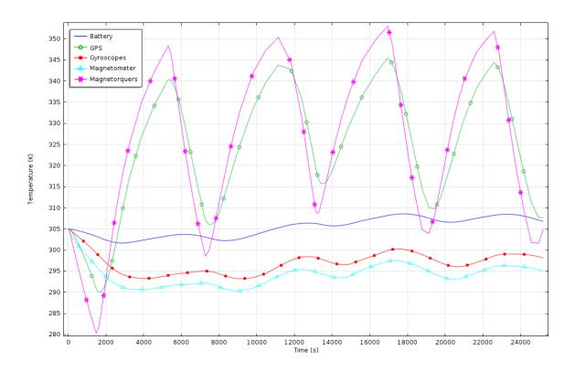
Figure 85: Average Temperature vs. Time for Components
