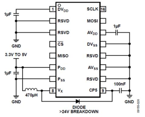
Gyroscope Application Circuit [80]
