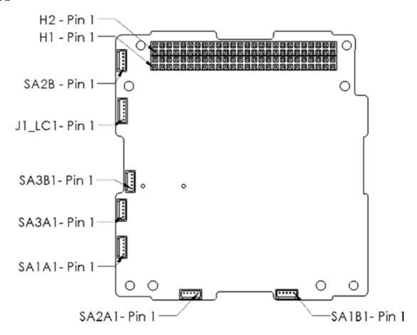
EPS Solar Array & CubeSat Header Connections [23]
