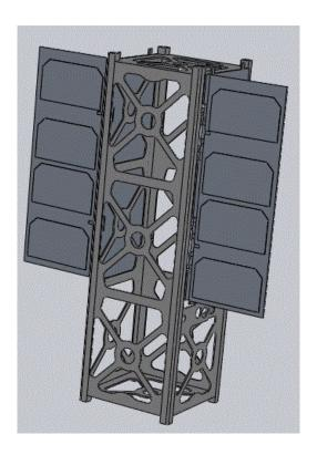
Figure 38: MQP Simplified External Structure
