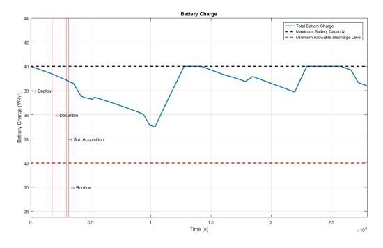
Figure 73: Battery Charge (Altered Sphinx-NG State Vector)
