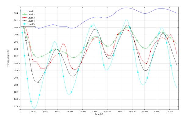
Figure 84: Average Temperature vs. Time for Circuit Boards
