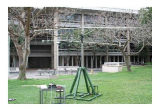
**Figure 27:** Built University of Hawai'i at Manoa Mobile Ground Station [50]
