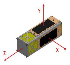
Figure 32: CubeSat Body Coordinate System Using the RHR [1] Copyright © 2013 WPI
