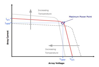
Figure 6: Solar Array Current vs. Voltage [23]. Copyright © 2016 Clyde Space Ltd.
