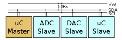
Figure 4: Inter-Integrated Circuit Bus [17] Copyright © 2016 I2C Info
