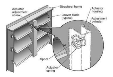
Figure 15: Schematic of Louver Assembly [42] Copyright © 2002 AIAA
