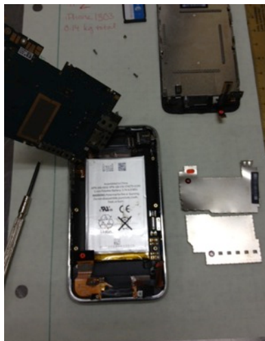
Figure 5. Liberation of PWB and SIM Card
