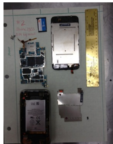
Figure 6. Step 5 - Removal of PWB
