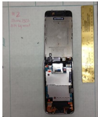
Figure 2. Step 2 - Separation of Front and Back Casing
