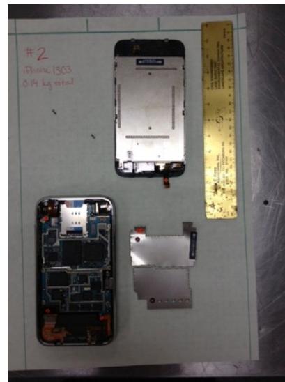
Figure 4. Step 4 - Removal of EMI Shield
