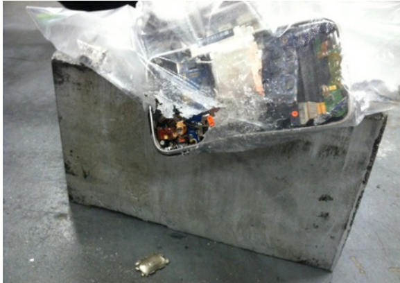
Figure 9. Partially Shredded iPhone 3
