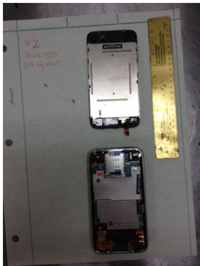
Figure 3. Step 3 - Complete Separation of Front and Back Casing
