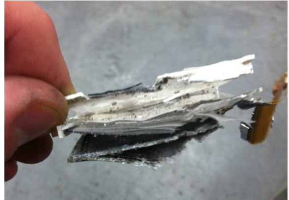
Figure 8. Layers of Shredded LCD Backing
