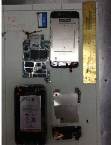
Figure 7. Step 7 - Removal of Bottom Connector
