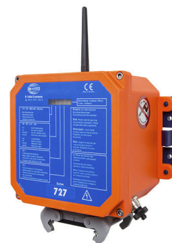
Figure 10 Onboard Receiver FSE-727 ( E-ONE, 2017)
