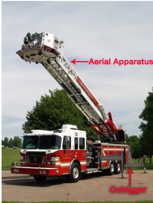
Figure 7 Aerial Apparatus and Outrigger (Fire Apparatus & Emergency Equipment, 2012).
