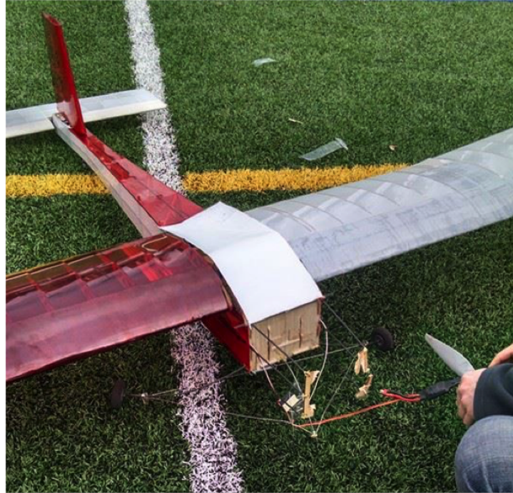
Figure 6.1: Damage Sustained during hops
