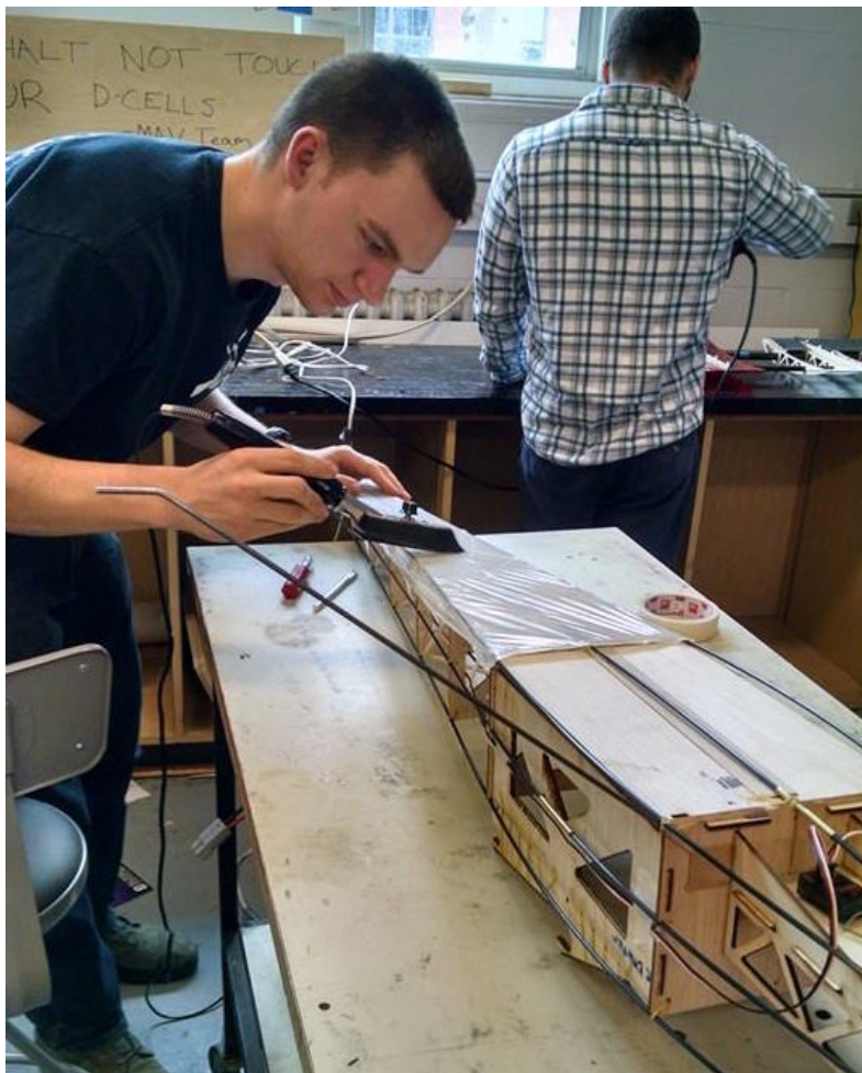
Figure 5.2: Coating the fuselage
