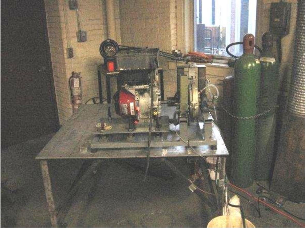
**Figure 2: Engine Dynamometer Test Stand**
