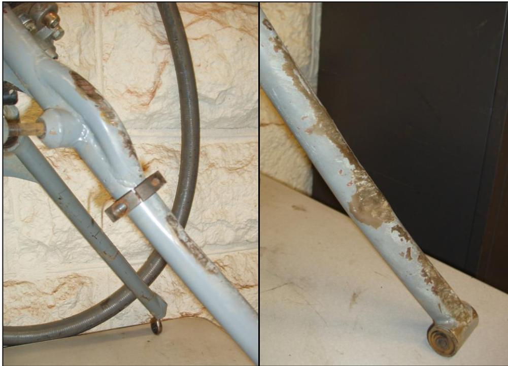
**Figure 34: Damage to Left and Right Lower Control Arms**
