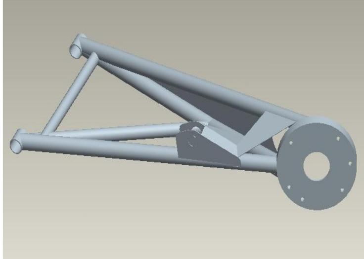
**Figure 20: 2007 Manufactured Trailing Arm**
