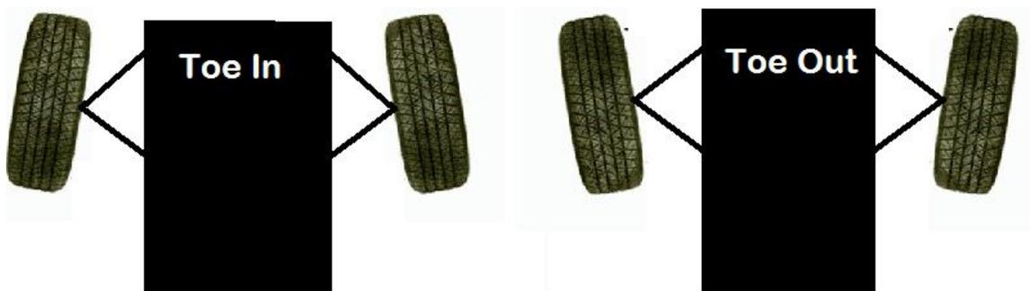
Figure 18: Toe-In and Toe-Out
