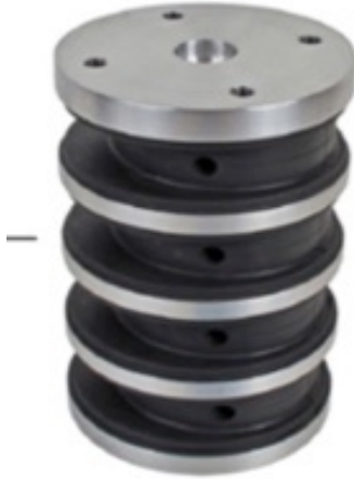
Figure 15: Hybrid III neck used as a guide for our manufactured neck
