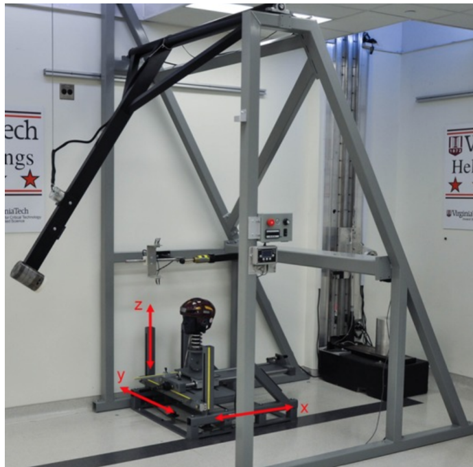
Fig. 8: Virginia Tech pendulum testing mechanism (Rowson et al., 2015)
