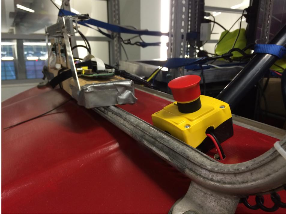
**Figure 5.22: Emergency switch located at the front of the vehicle.**
