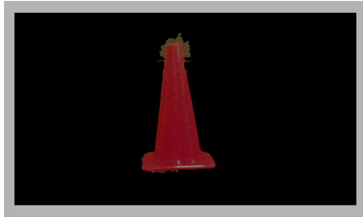
**Figure 7.10: The image data processed by the custom blob detection function displays only orange blobs currently within the view of the camera.**
