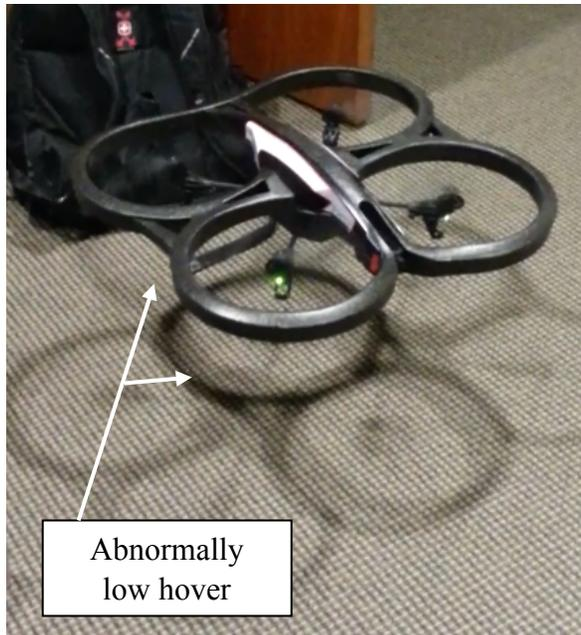
**Figure 7.3: Abnormally low hover height caused by reflection of ultrasonic pings and non-solid surfaces.**
