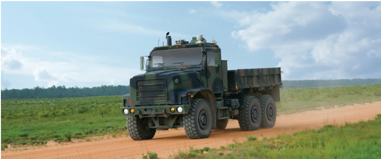
**Figure 2.2: The Oshkosh TerraMax Vehicle. This vehicle was designed to navigate extreme terrain, and comes equipped with a Velodyne HDL-64e Lidar module. The TerraMax also has wheels that can automatically change tire pressure to best suit its driving environment. This vehicle is capable of autonomous convoy driving [10].**
