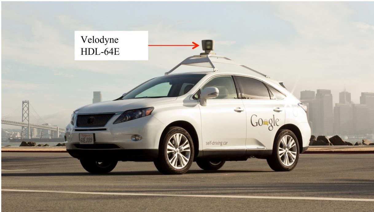
**Figure 2.4: The Google Car equipped with the Velodyne HDL-64e Lidar Module [13].**
