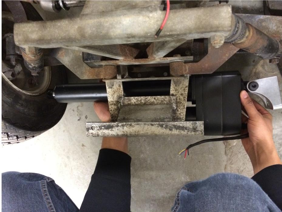
**Figure 5.3: The 560 lb linear actuator being held underneath the front bumper, with the actuator arm nearing the mounting point. The actuator barely fits and since there still would need to be a connection piece from the actuator to the steering rack, was deemed too large for use.**
