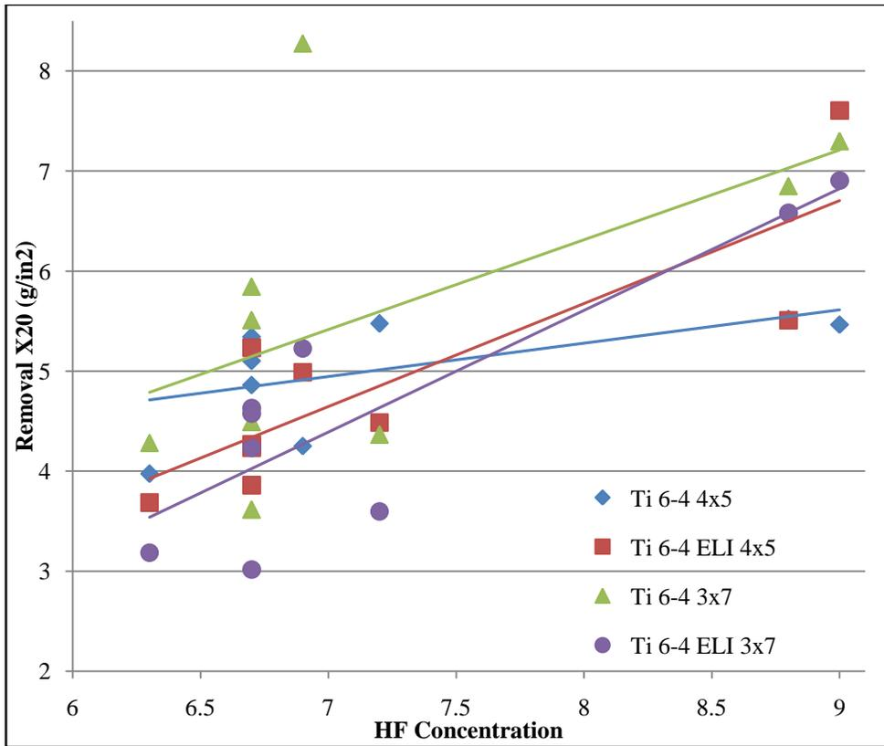
Figure 6: Metal Removal Dependence on HF Concentration
