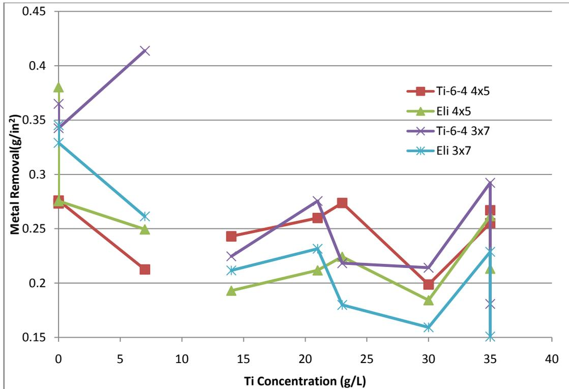
Figure 7: Metal Removal Dependence on Ti Concentration
