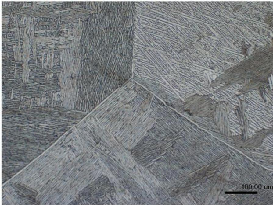
Figure 33: Ti-6-4 ELI, 10X Magnification
