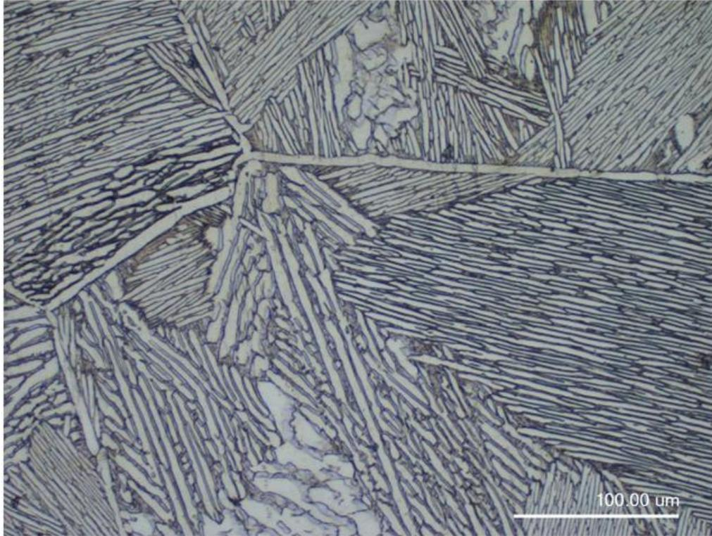
Figure 38: Ti-6-4, 20X Magnification
