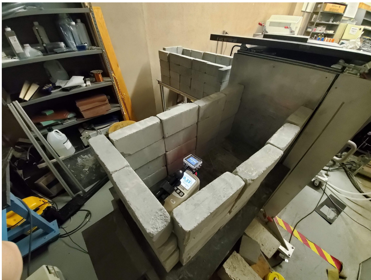
Figure 1: The collimator built in front of WPI's neutron generator, as seen from above. The ion chamber can be seen resting within the collimator. The concrete structure in the background of the picture is the side collimator; note the front collimator rests on a tabletop made of borated concrete, while the side collimator's table is aluminum.
