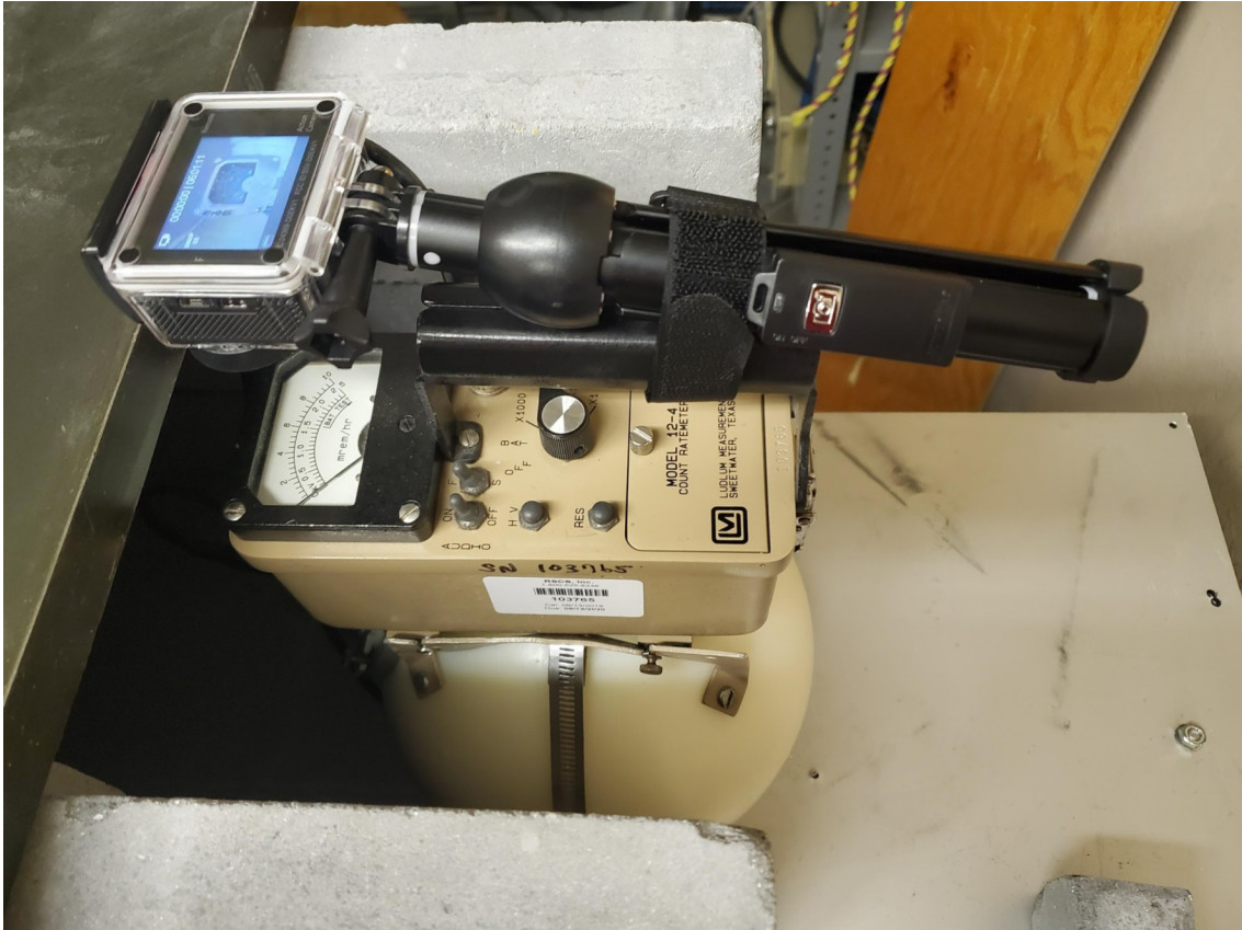
Figure 2: The GoPro camera, attached to the handle of the remball with a velcro strap. The camera is aimed at the display of the remball, allowing its measurements to be recorded while the operator is outside of the room and unable to read it.
