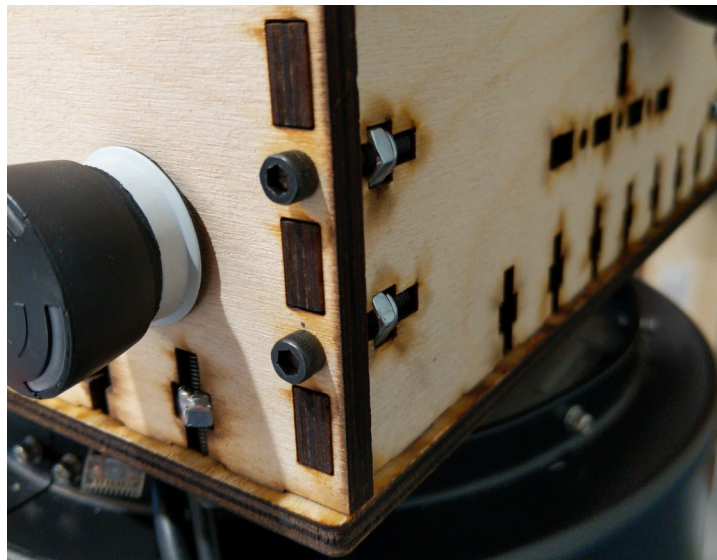
Figure 6 - Tab-Slot-Nut-Bolt Construction Strategy
