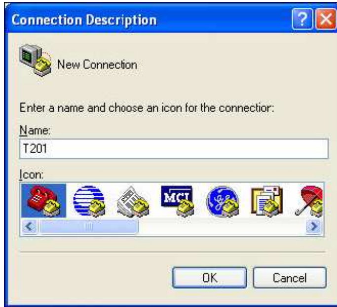
Figure 29: Dialog box to name the connection to the T201 RFID tag using HyperTerminal
