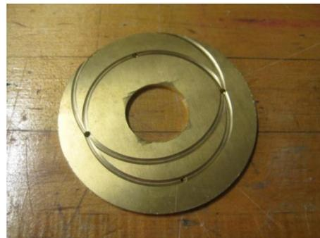
Figure 10: Machined Cam Bushing
