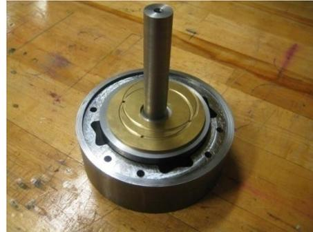
Figure 13: Carrier, Cam, and Cam Bushing
