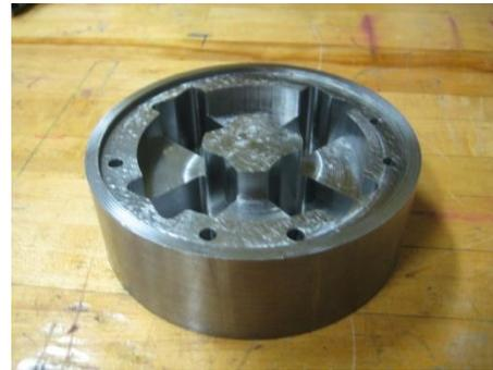
**Figure 7: Machined Side of Carrier**
