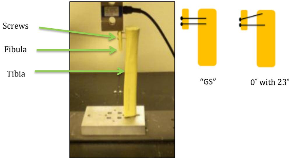
**Figure 5-6: Cyclic Shear Screw System Angles**
