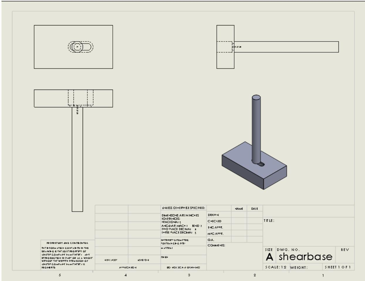
Figure 0-4: Test Rig for Shear Testing
