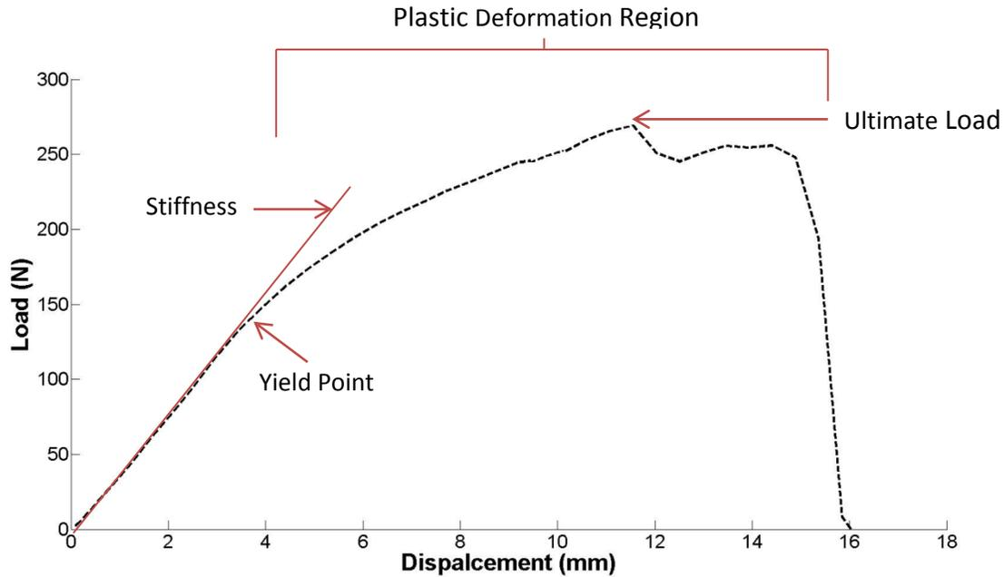
Figure 7-1: A representative plot from straight angled screw load-to-failure.
