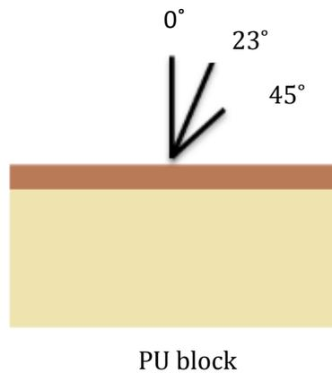
**Figure 5-2: Angles used for pullout testing**
