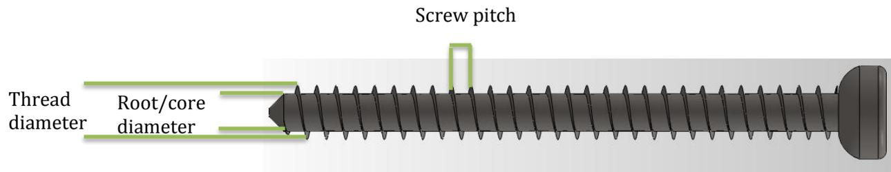
Figure 2-5: Bone Screw with Labeled Components
