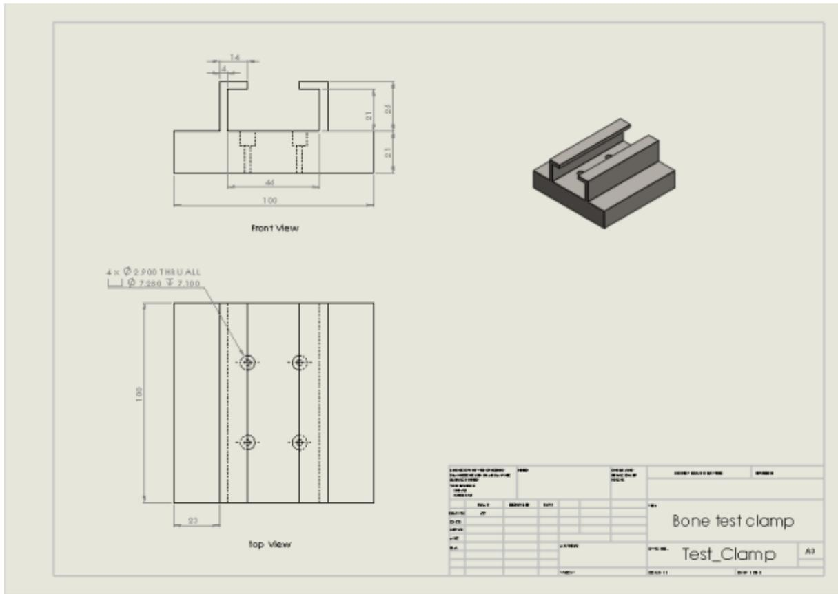
Figure 0-3: Test Rig for Pullout Testing
