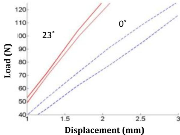
**Figure 6-3: Elastic Region of Load-to-Failure Testing**
