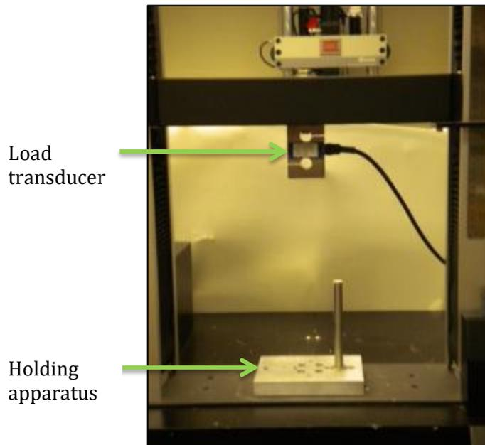
**Figure 5-4: Test Set-Up for Shear Testing**
