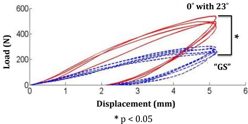
**Figure 6-5: Load-Displacement Graph of a Single Cycle of Cyclic Shear Testing**
