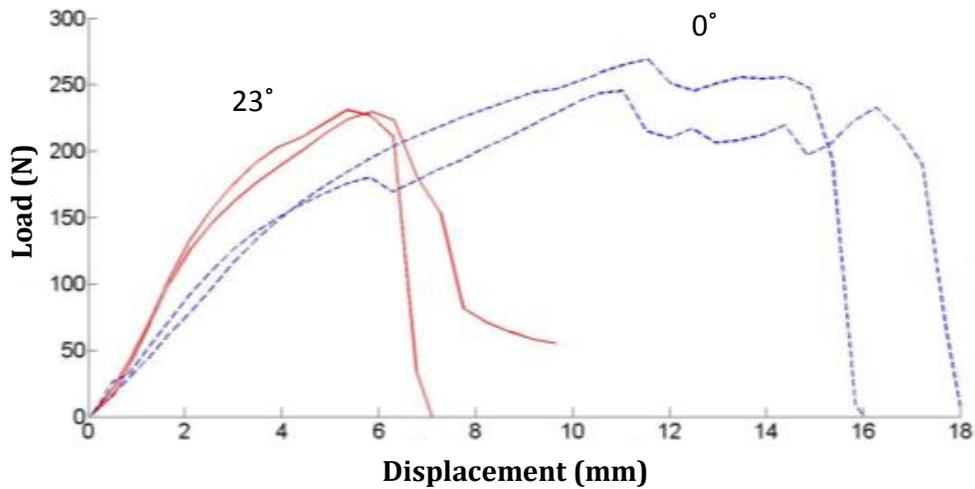
**Figure 6-4: Load-Displacement Graph for Load-to-Failure Testing**
