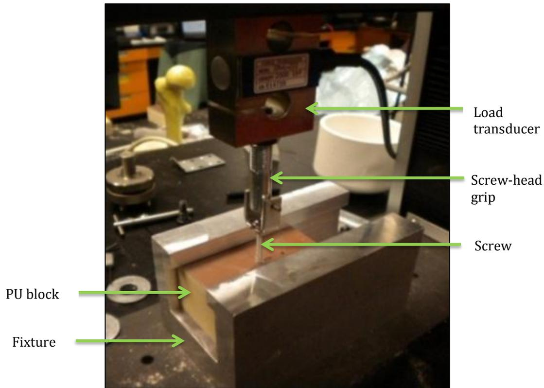
**Figure 5-3: Pullout Test Set-Up**
