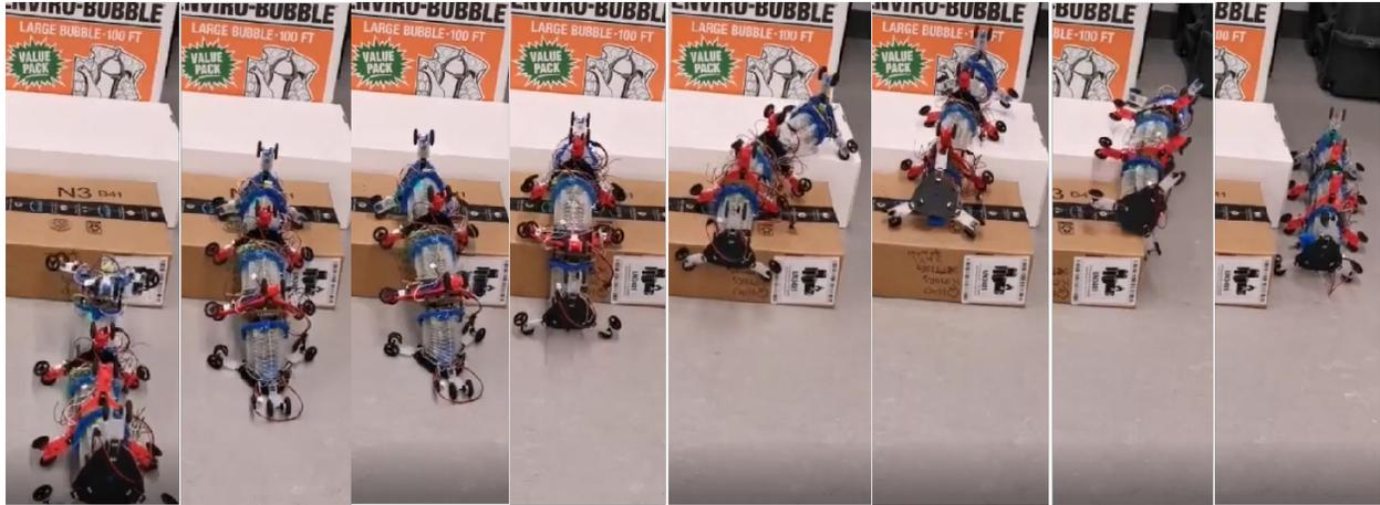
**Figure 3.18:** A 3 module salamander robot climbing over a 15 cm high obstacle.
