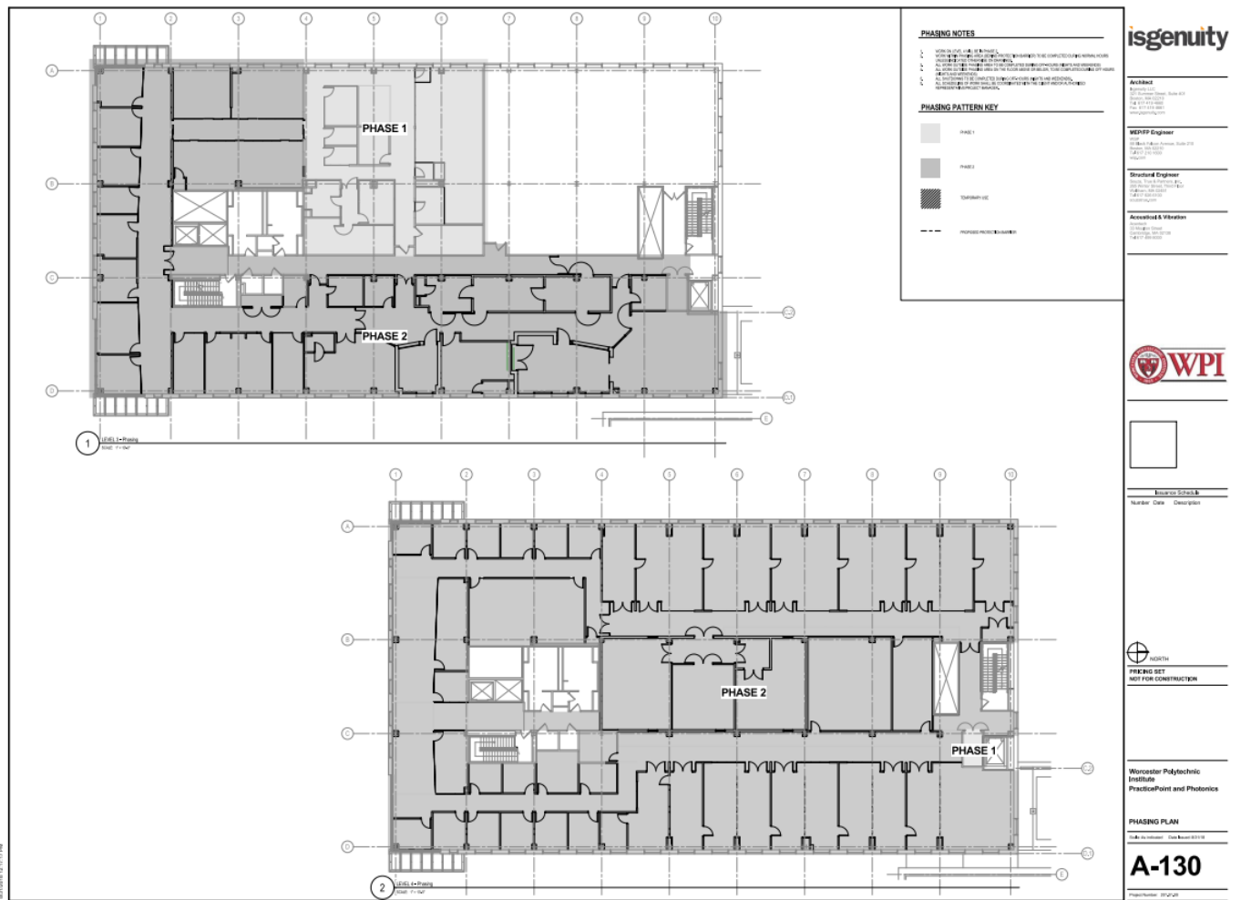
Figure 4: Phasing Plans for the third floor (top left) and the fourth floor (bottom right) of the Gateway II Renovation.
