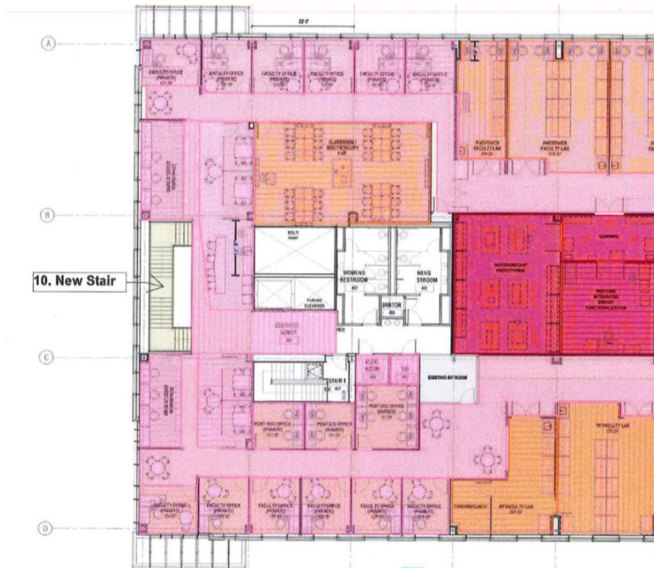
Figure 28: SD drawings showing the original staircase design.
