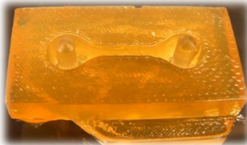
Figure 33. The final agarose mold with the PDMS posts going through the mold. A small PDMS base exists under the agarose mold that is attached to the posts in order keep the posts sturdy.
