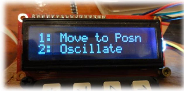
Figure 19. Stepper motor mode functions as displayed on the LCD main menu.
