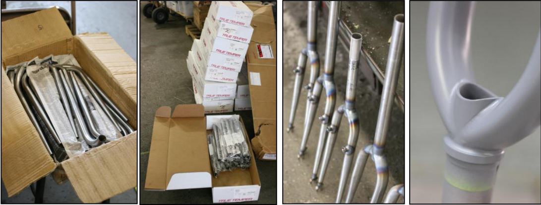
Figure 2-3 : Fabrication Process. From Left to Right: Fork Blades Arrive in Box, Steerer Tubes Arrive in Box, Parts are Welded, Forks are Primed and Painted.
