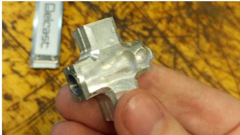
*Figure 7.10: Warped Block Joint*
