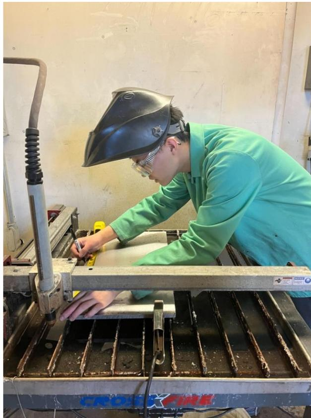
*Figure 24.20: Brendyn Lining Stock into Plasma Cutter*
