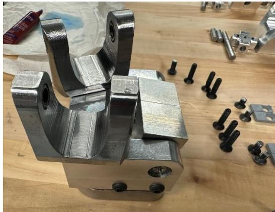
*Figure 8.3: Connection between the Ankle block, Ankle Roll Actuation Link, Ankle Pitch and Roll Coupling, and Bottom Joint Connector V3*
