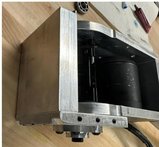
*Figure 8.31: Attaching BS2 Piece 3 to BS2 Piece 2 with M5 Countersink Screws*
