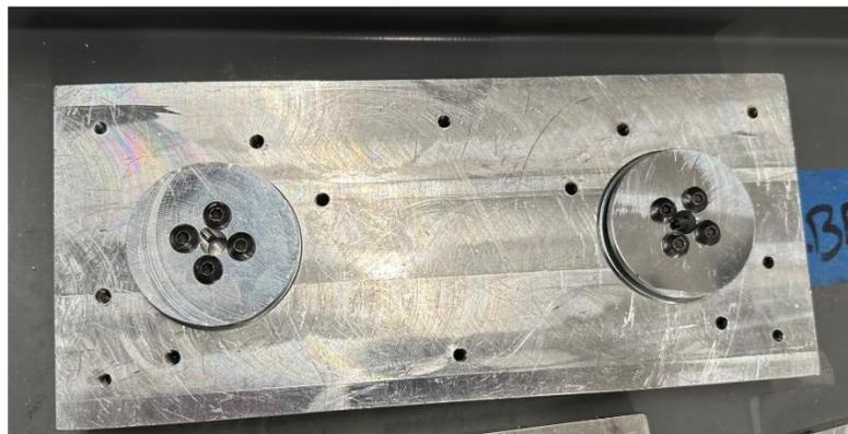
*Figure 8.44: Screwing the Hip Yaw Mount Top/Bottom together with M5 Button Head Screws*
