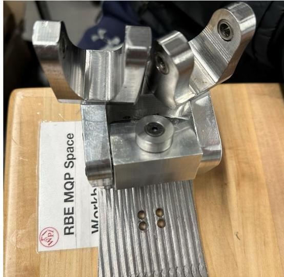
*Figure 8.7: Attaching Bottom Mount of Rotational Adjustment to the back of the Ankle Roll Coupling*
