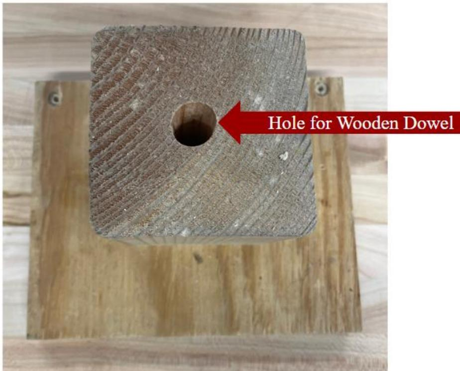
Figure 6.10: Bottom Part of Weighing Mechanism (Top-View)
