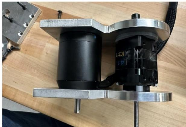
*Figure 8.36: Attaching Bracket Stage 1 Out to the gearbox*
