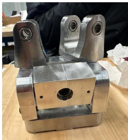
*Figure 8.4: Front view of connection between the Ankle block, Ankle Roll Actuation Link, Ankle Pitch and Roll Coupling, and Bottom Joint Connector V3*
