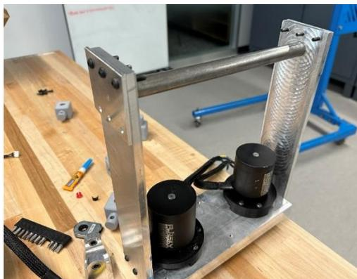
*Figure 8.49: Screwing Plates onto the Test Rig Side Plates*
