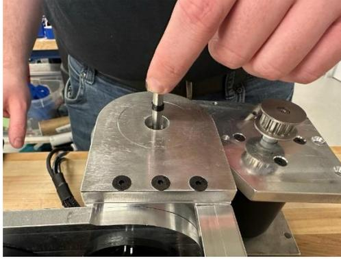
*Figure 8.39: Attaching BS2 Piece 2 to BS2 Piece 2 and on Bracket Stage 1 In with M5 Countersink Screws*
