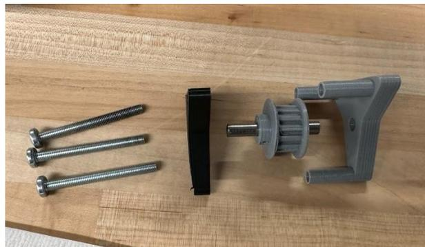
*Figure 8.24: Layout for assembling a tensioner for the pulleys*
