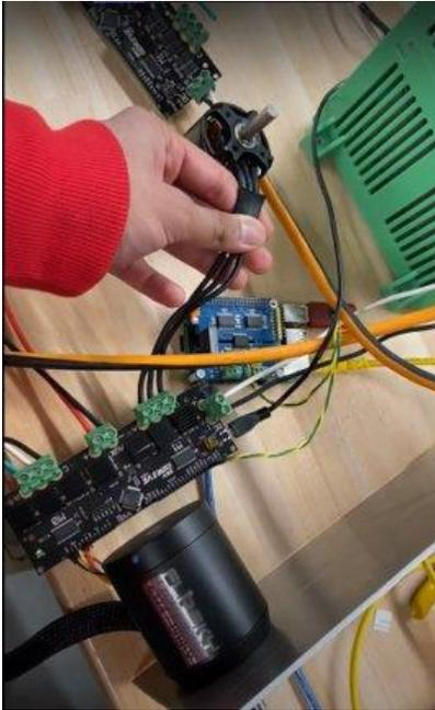
*Figure 12.2: The benchtop CAN bus test setup*
