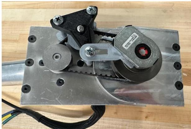
*Figure 8.34: Attaching the tensioner and belt*
