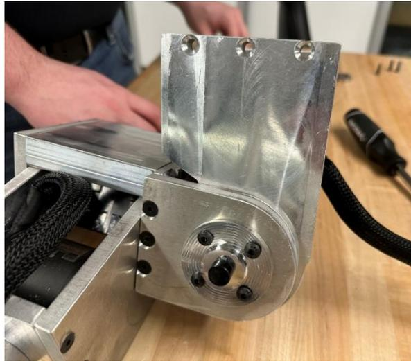
*Figure 8.38: Attaching a Knee Output Shaft Connector to BS2 Piece 1 with M5 Button head Screws*
