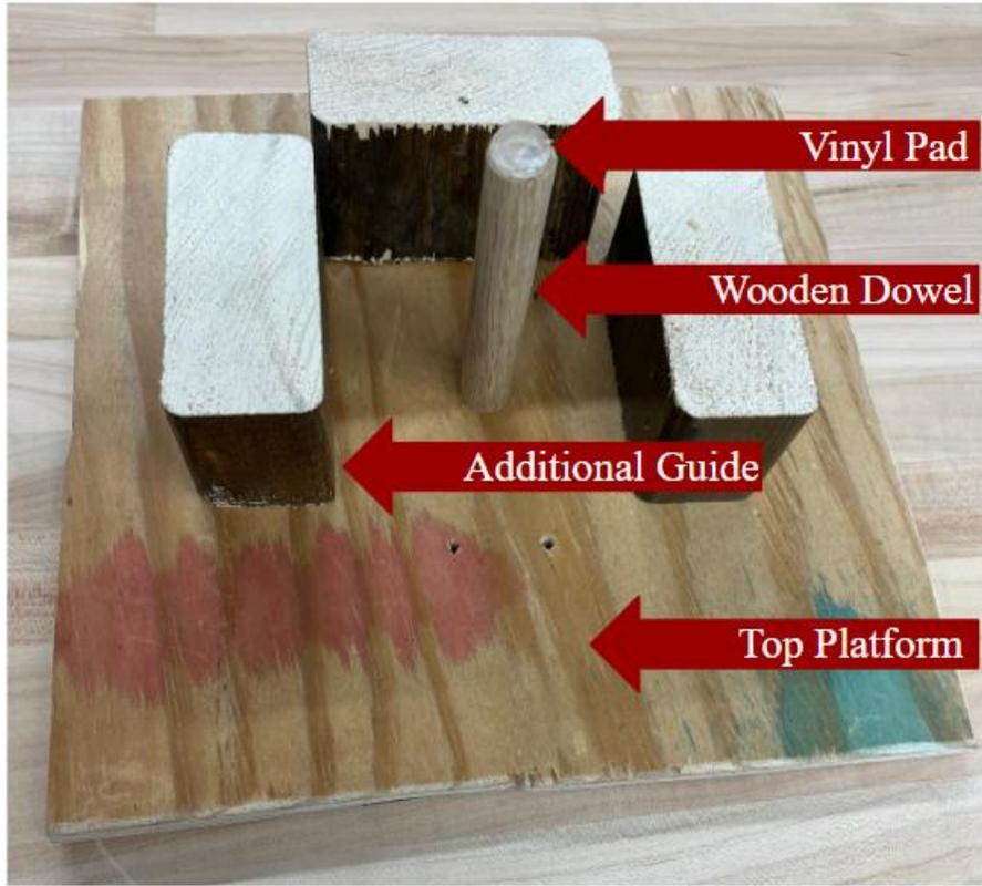
Figure 6.9: Top Part of Weighing Mechanism (Up-side Down)
