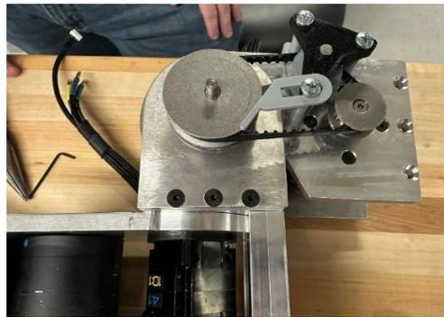
*Figure 8.40: Attaching the pulleys and tensioner*
