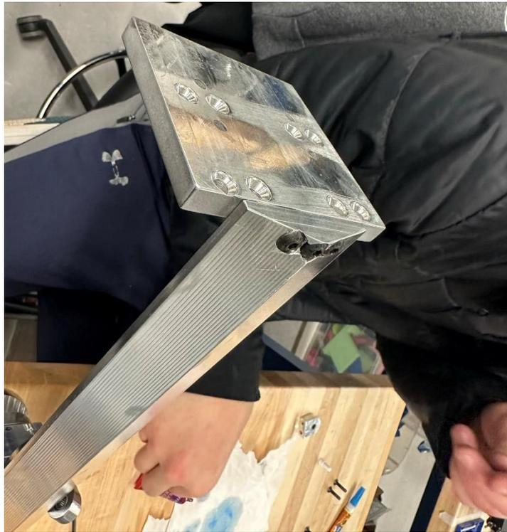
*Figure 8.9: Attaching Ankle Top Plate to the top of the Ground Link with M5 Button Head screws*
