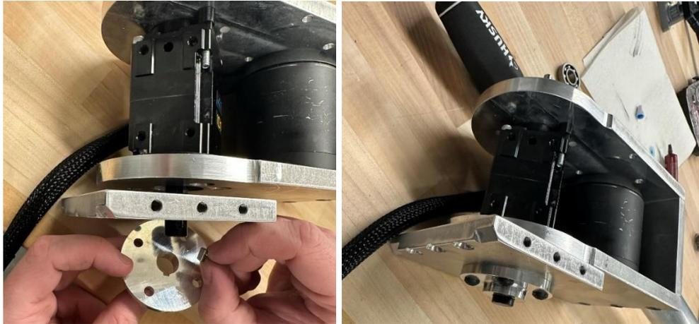
*Figure 8.30: Attaching a Knee Output Shaft Connector and BS2 Piece 2 to the Bracket Stage 3 Out (left) with M5 Button head Screws (right)*
