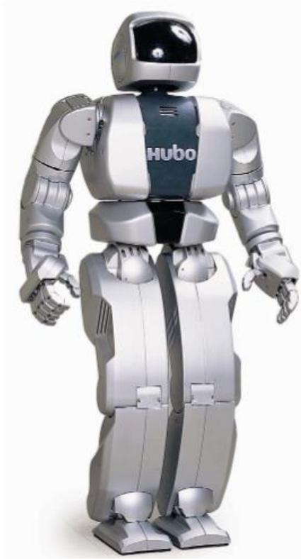
*Figure 3.19. The humanoid robot KHR-3.*
