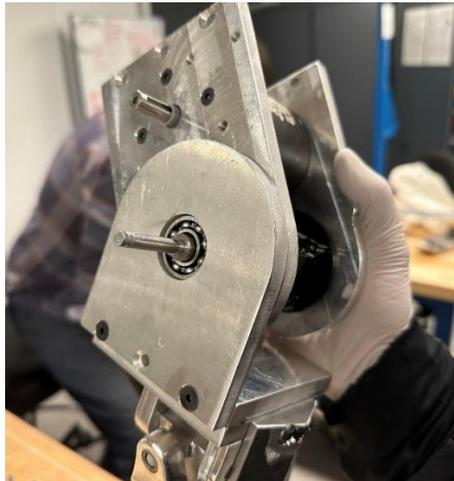
*Figure 8.20: Attaching Side Plate 1 to Side Bracket 1 using M5 Countersink Screws*
