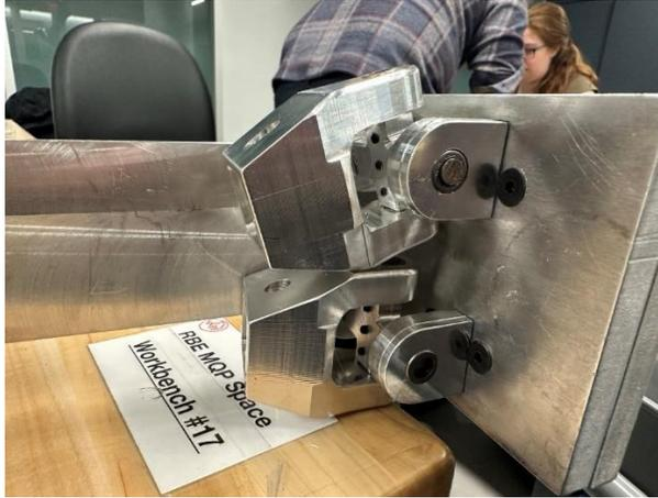
*Figure 8.14: Both Bottom Joint Connectors attached to the Ankle Top Plate U-Joint Attachments*
