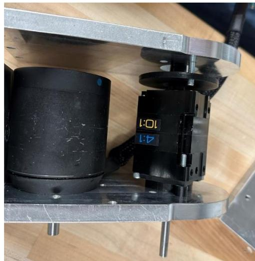
*Figure 8.29: Attaching gearbox to Bracket Stage 3 Out with spacer*
