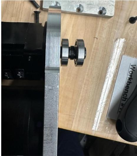
*Figure 8.19: Bearing and spacer layout that goes on the gearbox shaft*
