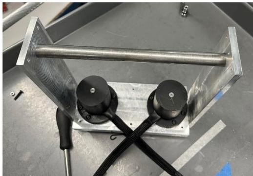
*Figure 8.48: Putting Steel Rod through the Test Rig Side Plates*
