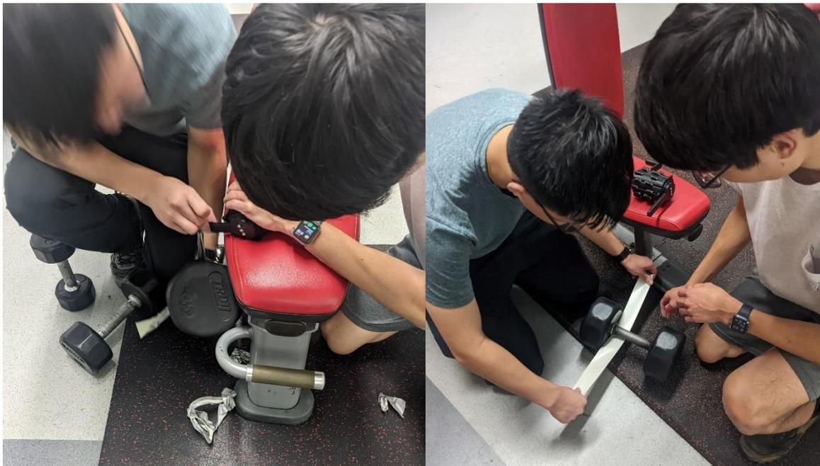
Figure 24.16. Brendyn and Jonathan attached the 35lb weight to the Harmonic Drive with duct tape.
