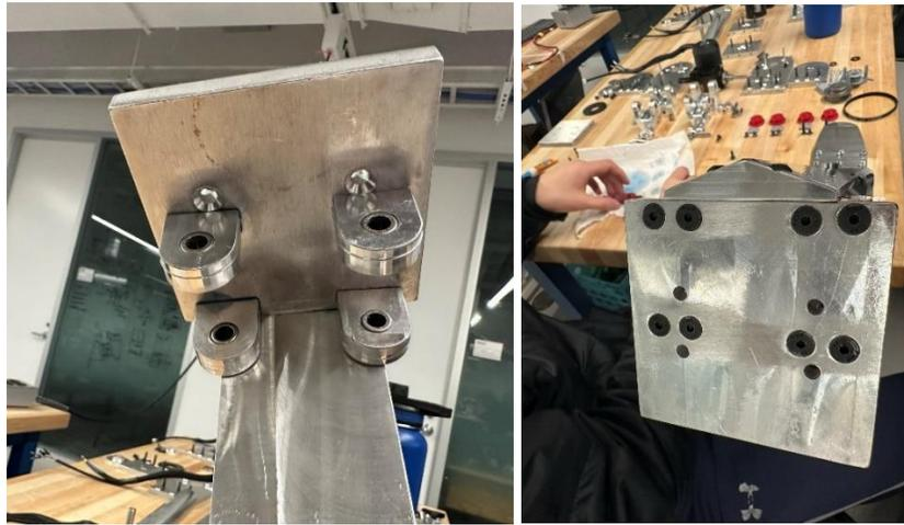
*Figure 8.10: Attaching 4 Ankle Top Plate U-Joint Attachments to the bottom of the Ankle Top Plate (Left) with M5 Countersink Screws from the top (right)*
