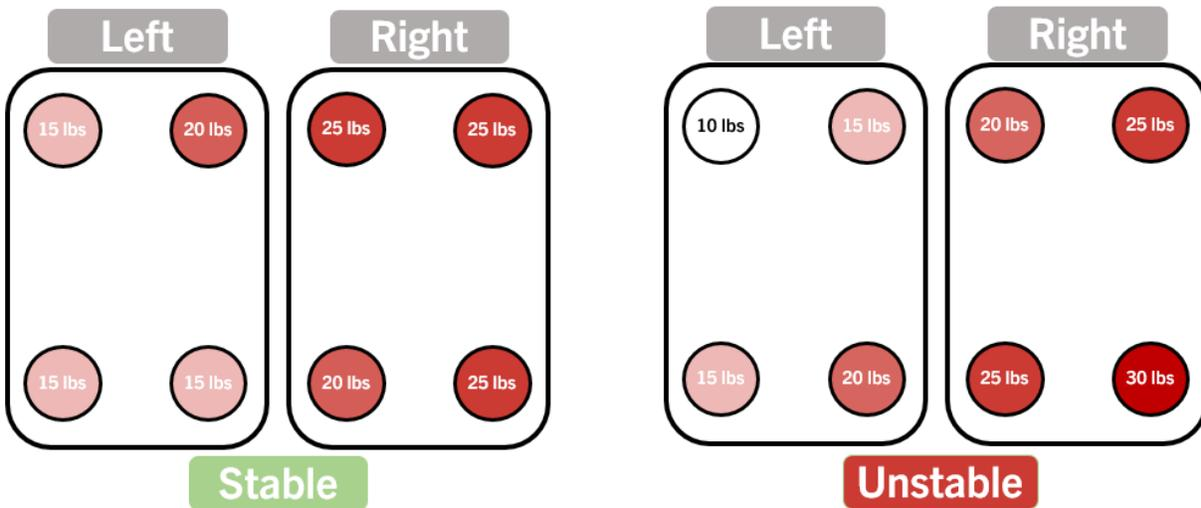
Figure 3.41: Theorizing a Stable and Unstable State From Reading Robot's FSRs
