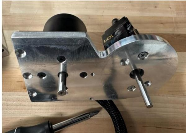
*Figure 8.35: Attaching a motor and gearbox to Bracket Stage 1 In*
