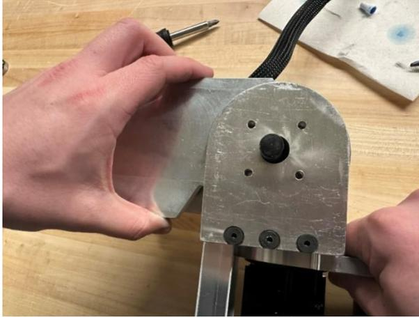
*Figure 8.37: Attaching BS2 Piece 1 to BS2 Piece 2, with Bracket Stage 1 Out to BS2 with M5 Countersink Screws*
