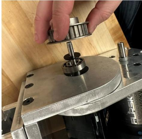
*Figure 8.23: Attaching a bearing, spacer, and large pulley on the gearbox input shaft*
