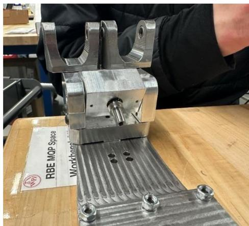
*Figure 8.6: Attaching shaft into the Ankle Roll Coupling*
