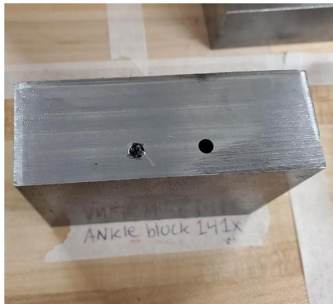
*Figure 7.11: Broken Tap (left hole) in Steel Part*
