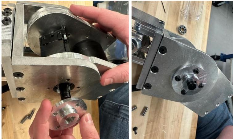
*Figure 8.22: Attaching the Knee Output Shaft connector with a key in the gearbox shaft (left) using M5 Button head Screws(right)*
