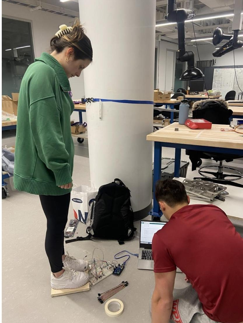
*Figure 6.25: FFSM data collection. FSRs were attached to the bottom of two pieces of wood, representing the left and right feet.*
