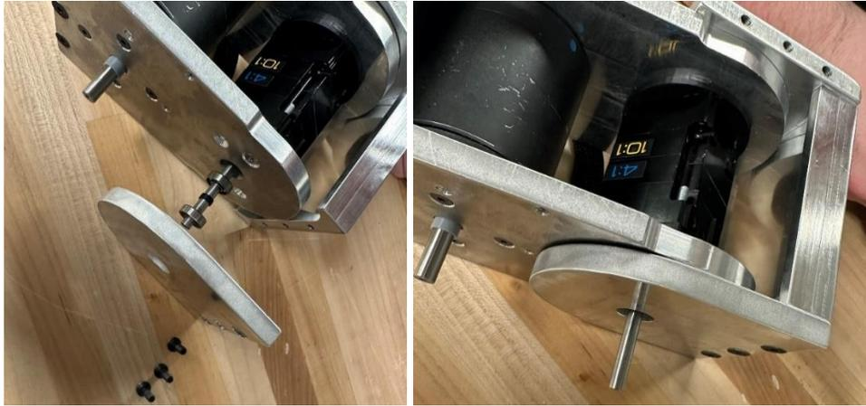
*Figure 8.32: Attaching a bearing, spacer, bearing, and BS2 Piece 1 to Bracket Stage 3 In (left) with M5 Countersink Screws (right)*
