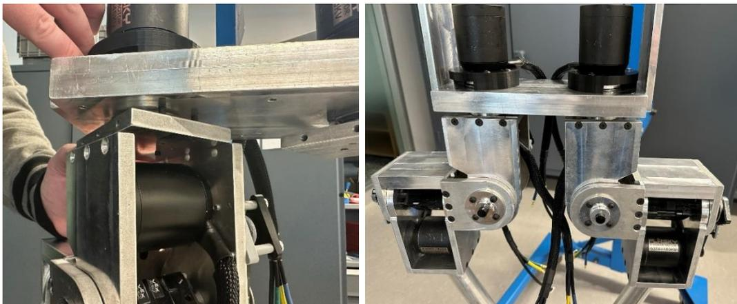
*Figure 8.50: Putting the Leg Assembly onto Bracket Stage 1 Top (left) with M5 Countersink Screws (right)*
