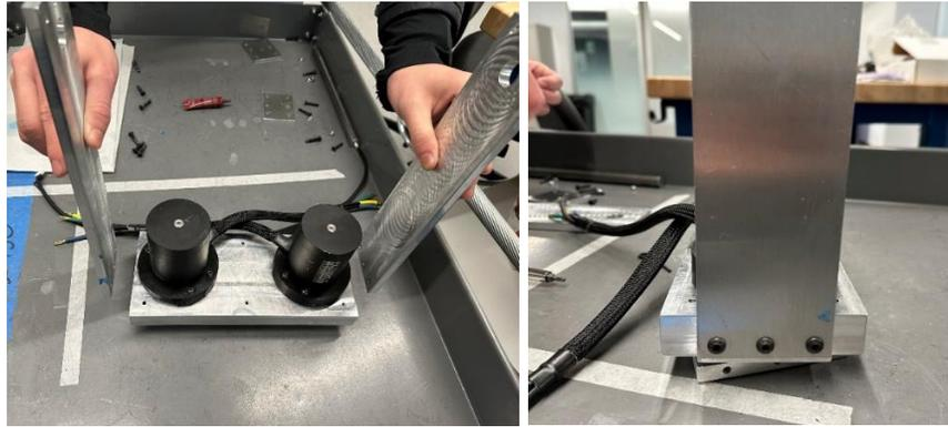
*Figure 8.47: Attaching Test Rig Side plates onto the pelvis (left) using M5 Button Head Screws (right)*
