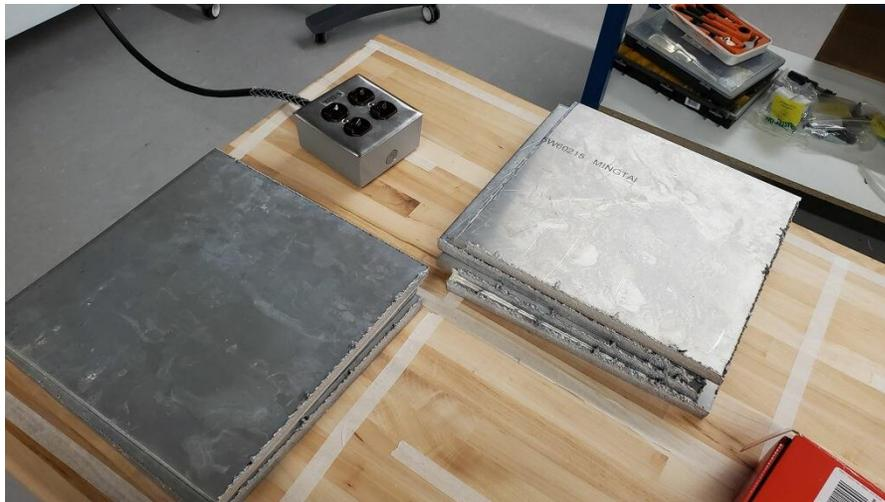
*Figure 7.13: Waterjet stock Cut to 1ft x 1ft*
