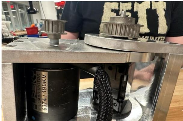
*Figure 8.33: Attaching both pulleys on Bracket Stage 3 In and BS2 Piece 1*
