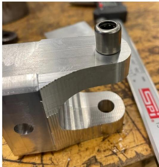
*Figure 7.12: Bearing Size Issue in Aluminum Part*
