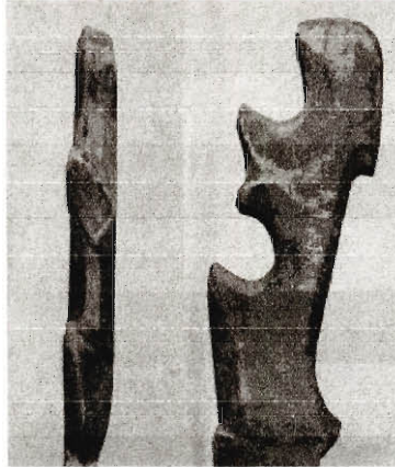
Figure 3: Front and side view of a 'work' fórcole
