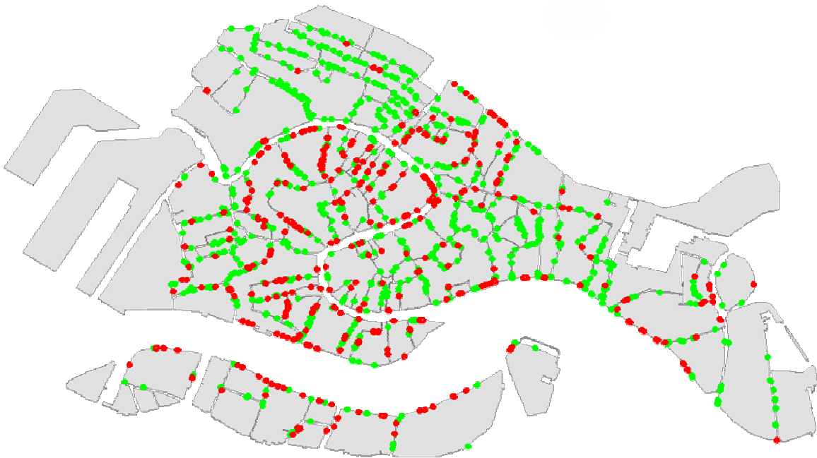
Figure 4-6: Usable (Green) and Unusable (Red) Docks
