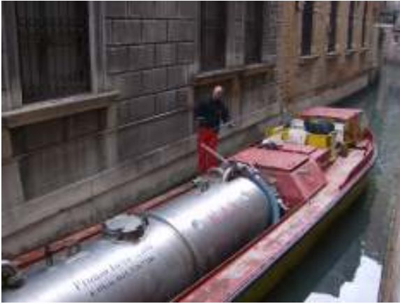
Figure 9: One of the sewage collection boats used to remove solids from sediment tanks
