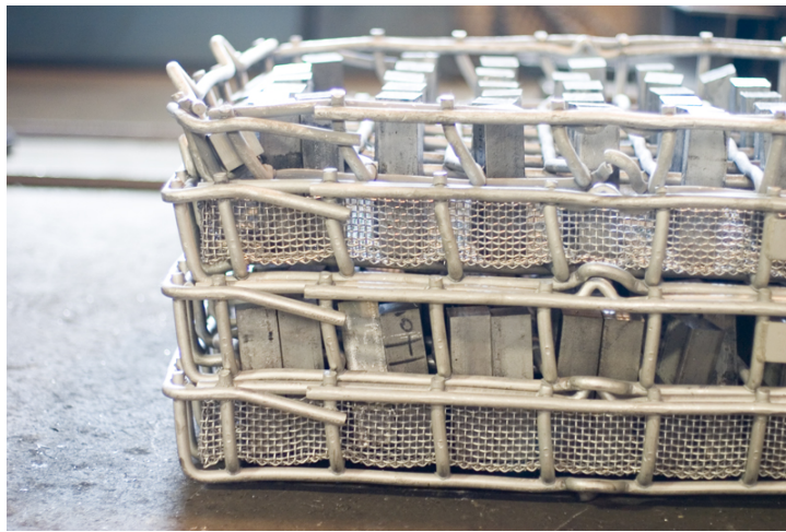
Figure 57. Arrangement of workpieces in the basket
