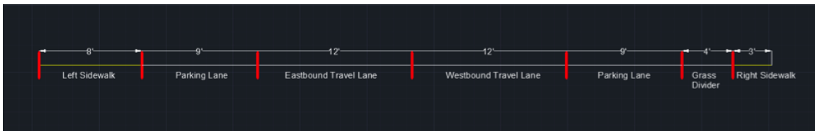
Figure 3: Existing Street Profile of Highland Street between Park Avenue and Newton Square
