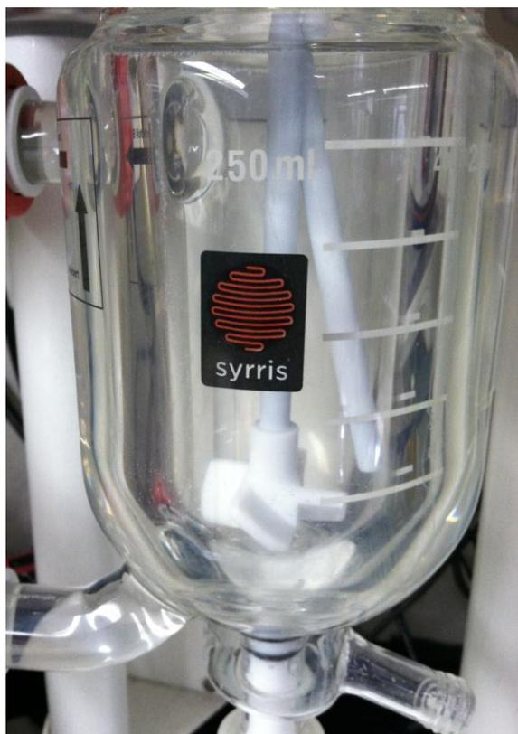
*Figure 6: Small reactor with a heating water jacket*
