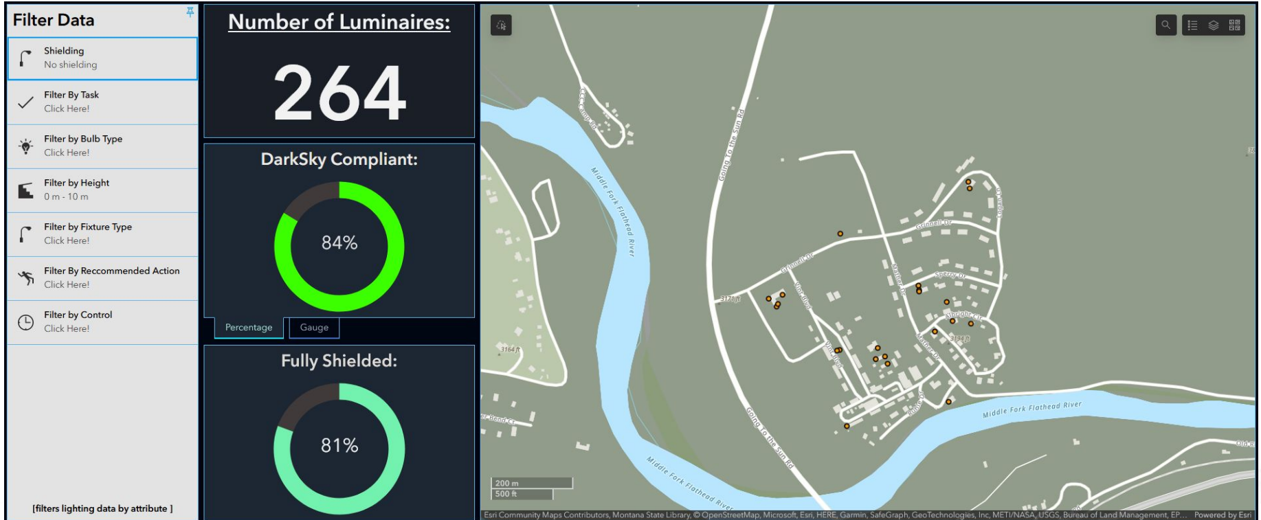
Dashboard screen and filter tab displaying the Headquarters area. Total number of luminaires, or light fixtures, on screen, dark sky compliance percentage, and percentage of fully shielded lights shown. The “No Shielding” option is activated, showing only lights with no shielding.
