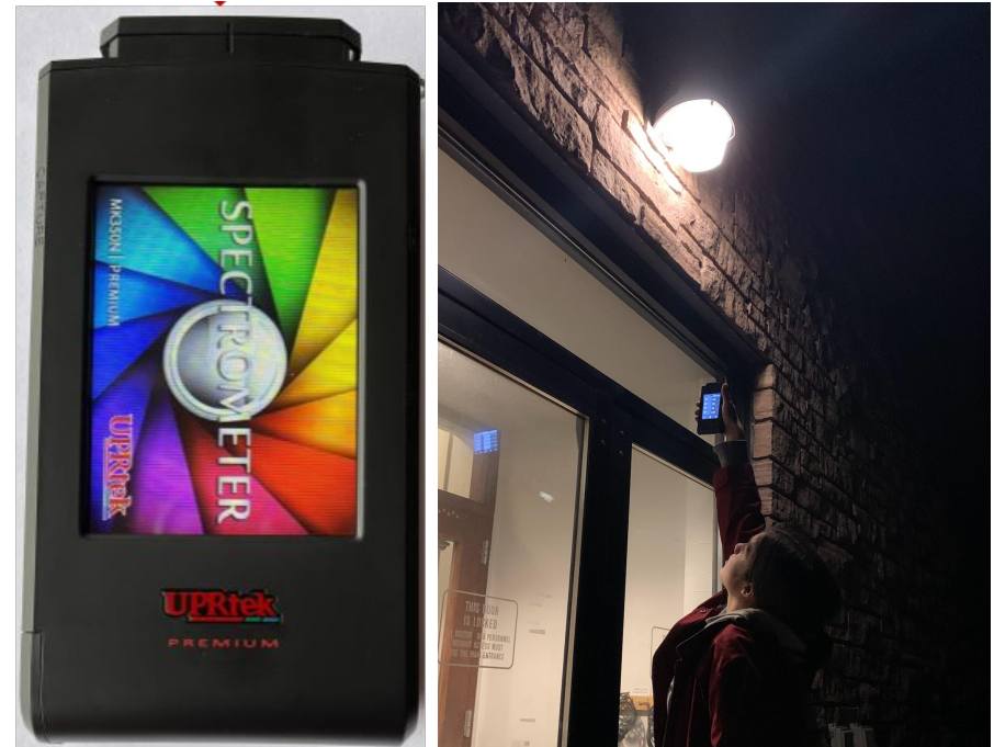
Figure 25. Spectrometer used to measure CCT (left). Measurements are required to be taken at night, pointing the sensor toward the light (right). Photos by Ryann Dionne.
