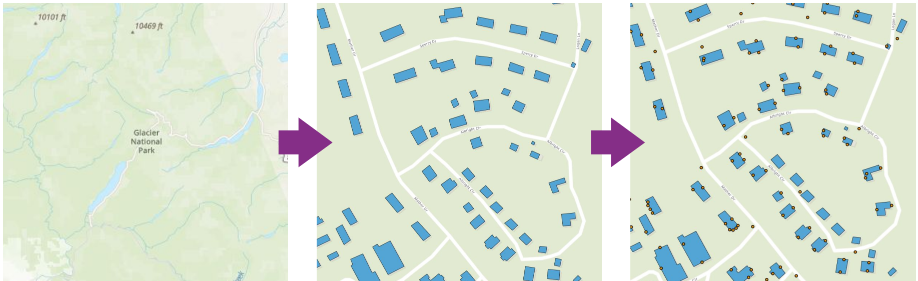
Figure 21. The lighting inventory map is composed of three layers: topographic world map (left), Glacier National Park building data layer (middle), and luminaire data layer (right). The luminaire data layer is where the lighting inventory data is logged.
