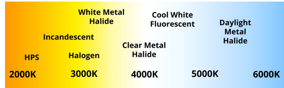
Figure 9. Examples of light bulbs and their respective color temperatures (DarkSky International, 2023b).
