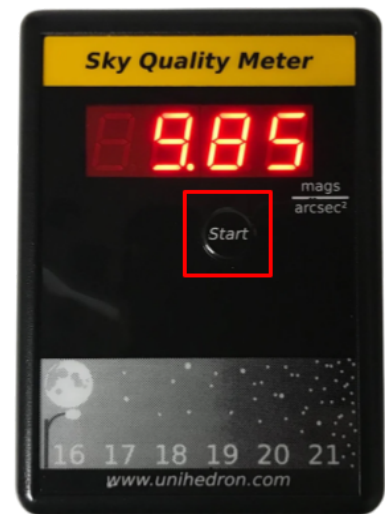
Front panel of the Sky Quality Meter with lens, the only control is the “start” button on the front [1].
