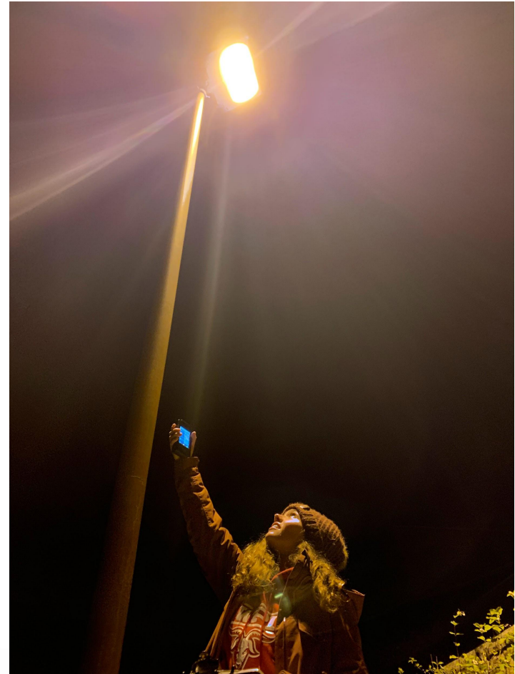
Figure 46. Taking a CCT measurement of a lamppost at night with a Spectrometer. Photo by Evan Dapsis.
