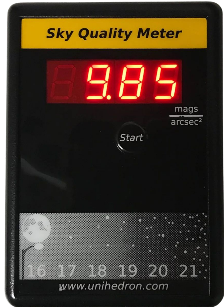
Figure 8. A Sky Quality Meter with lens, or SQM-L, displaying the recorded magnitudes per square arcsecond (mpsas) (Astronz, n.d.).
