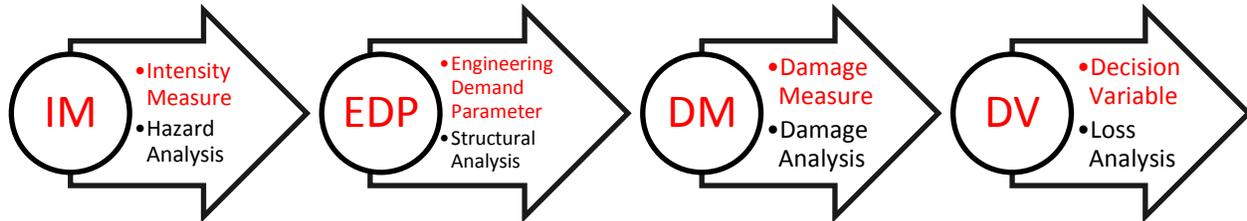
**Figure 6. PEER PBEE methodology process**
