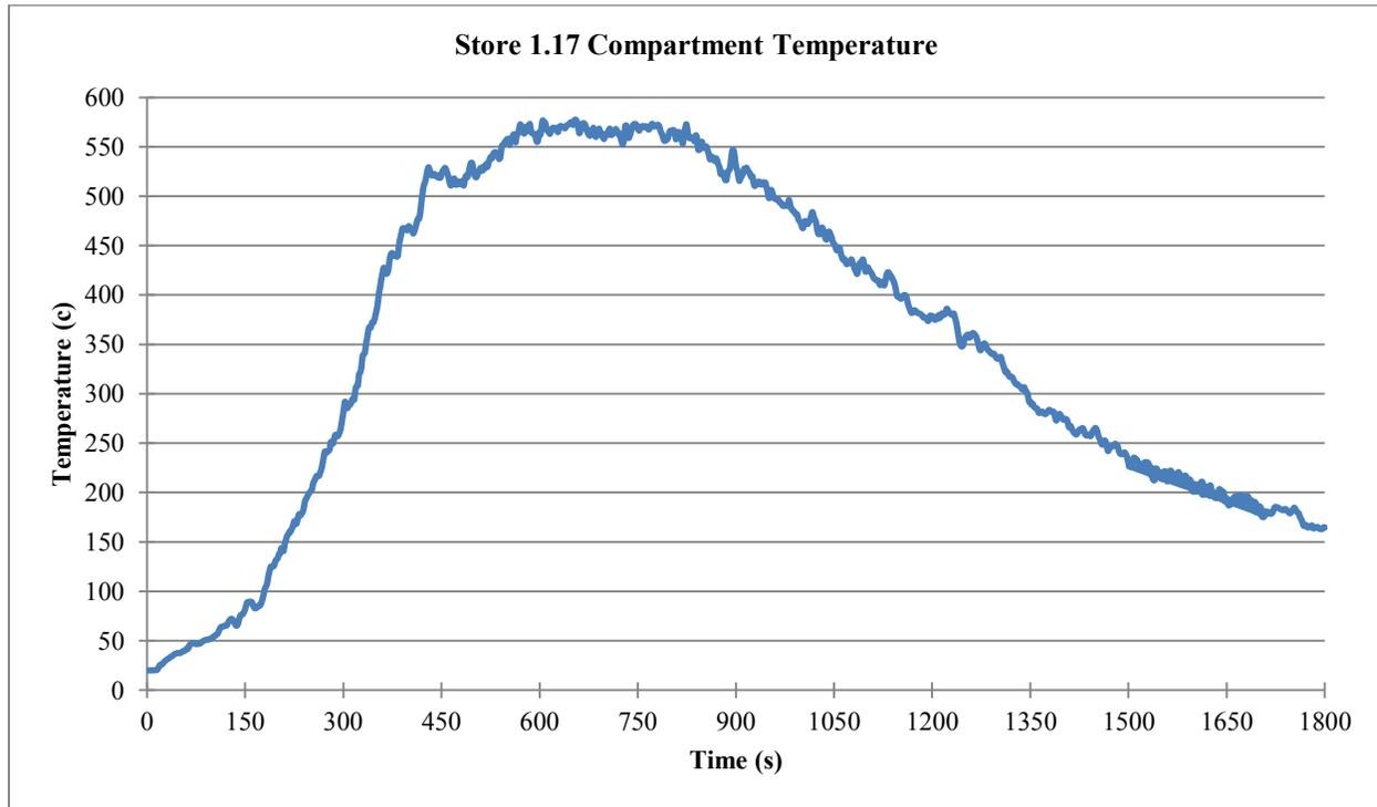
**Figure 72. Post-Earthquake building fire store 1.17 gas temperature at 2.8m height from floor**
