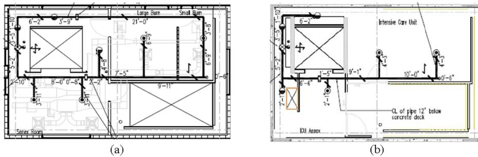
Fig. 5. Sprinkler system layout for (a) Floor 3 and (b) Floor 4 [10].
