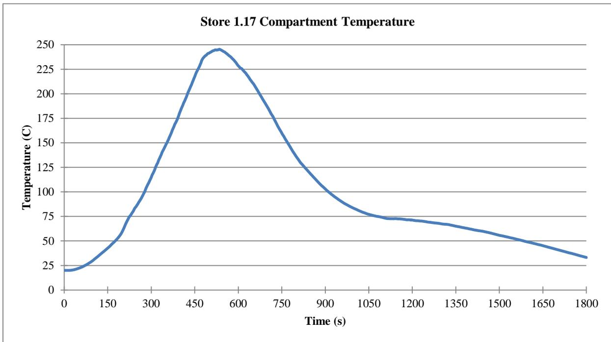
**Figure 52. WPI Mall store 1.17 gas temperature at 2.8m height from floor**
