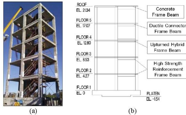
Fig. 2. Test specimen (a) skeleton; (b) elevation view (elevation in m) [images and schematic from 8].
