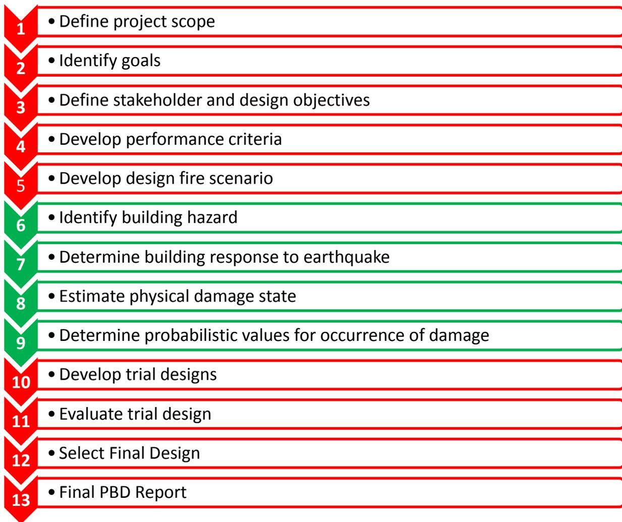
**Figure 91. Step-by-step procedure for conducting PBD on earthquake prone buildings**
