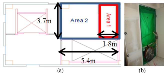
Fig. 14. Compartment integrity tests on Floor 3: (a) test areas 1 and 2 and (b) installation of blower door.
