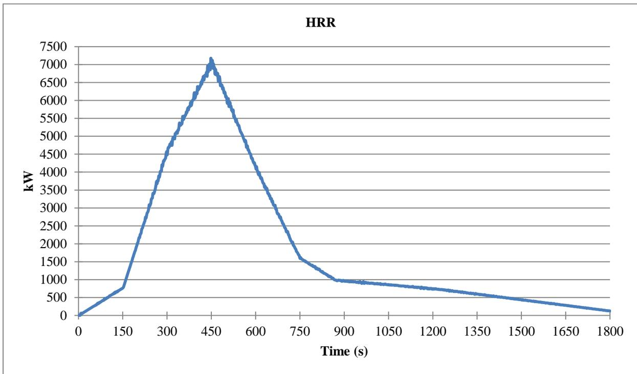
Figure 51. Normal WPI Mall HRR Curve
