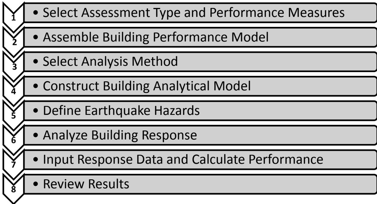
Figure 12. ATC-58 performance assessment process (ATC-58, 2012)
