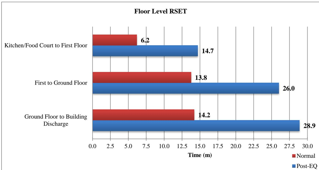
**Figure 88. Floor by floor occupant evacuation time**
