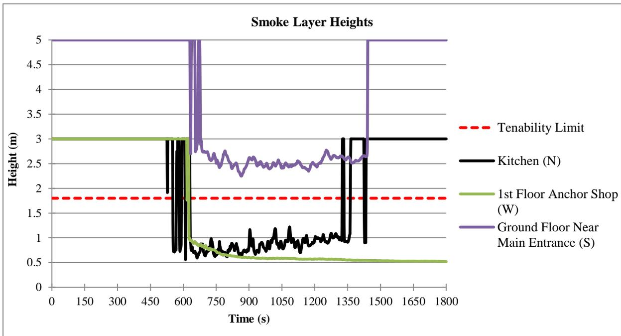
Figure 76. Post-earthquake fire Smoke Layer Heights at various locations
