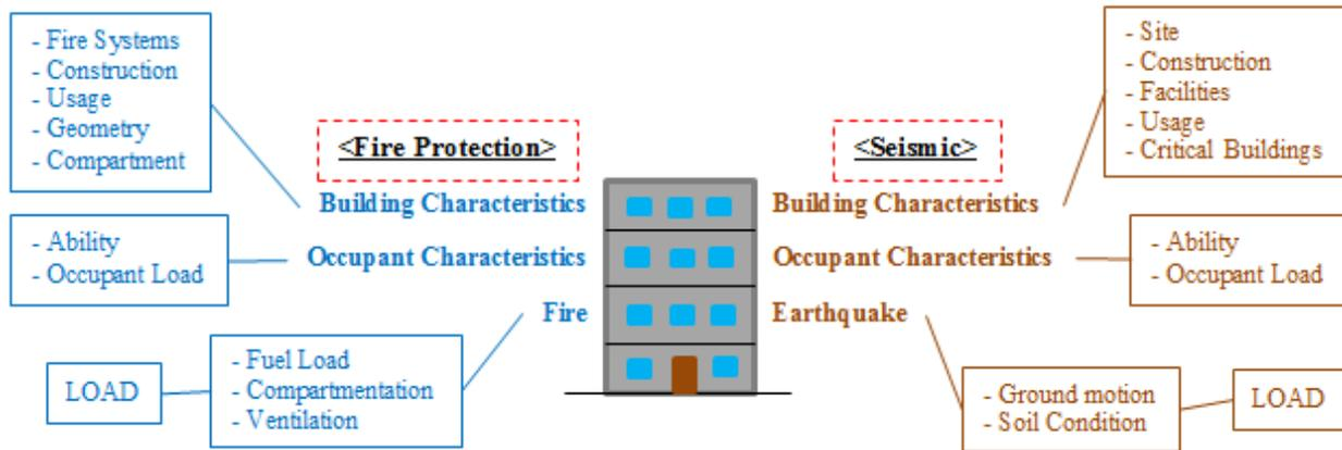
**Figure 13. Building features which can affect the design**
