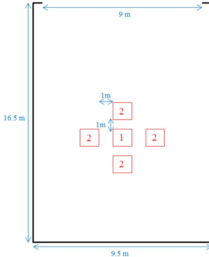
Figure 48. Set up of normal WPI Mall clothing fire in store 1.17
