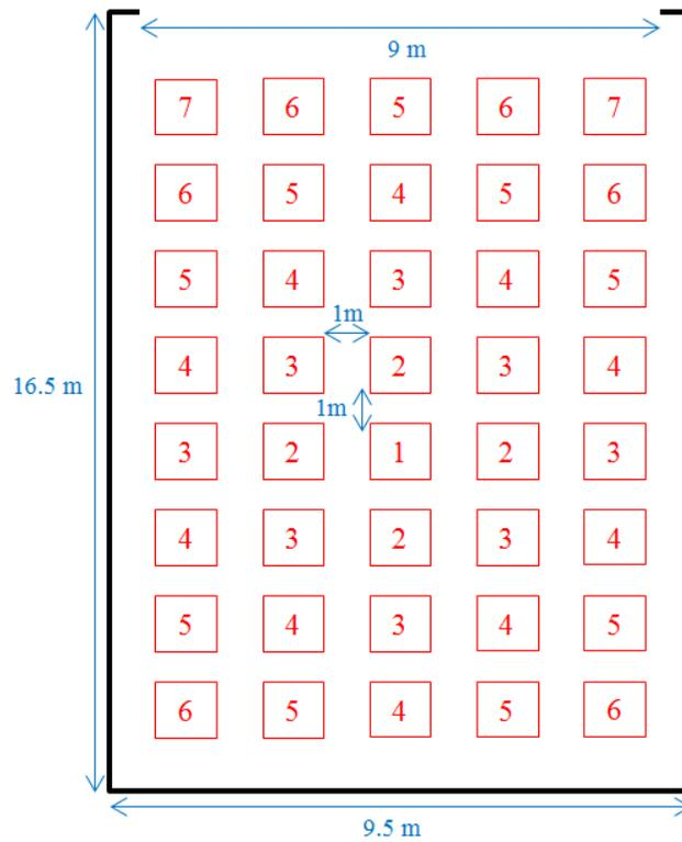
Figure 69. Set up of earthquake damaged WPI Mall clothing fire in store 1.17
