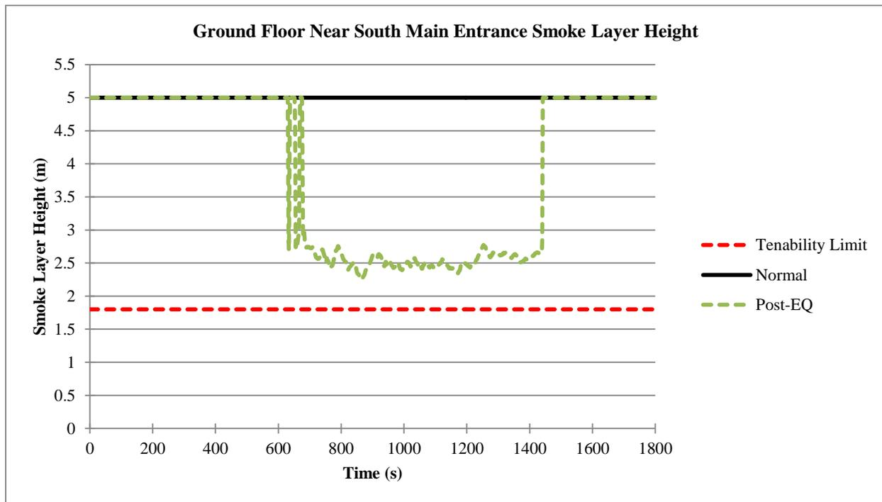
Figure 87. Smoke layer height comparison near the ground floor south main entrance
