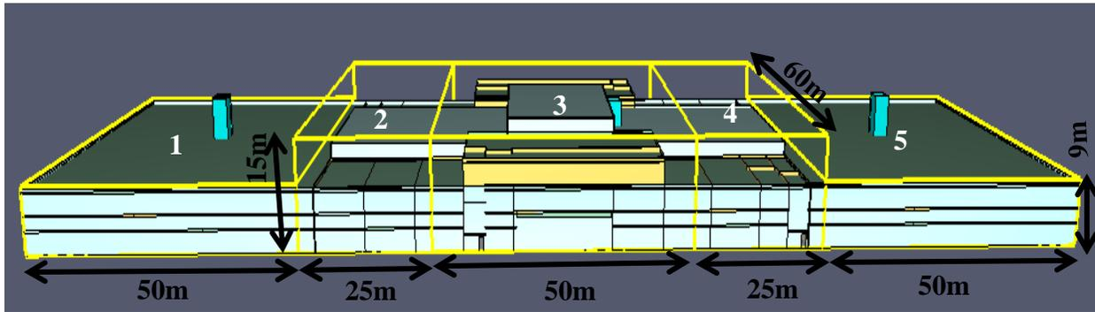
Figure 44. FDS computational domain setup
