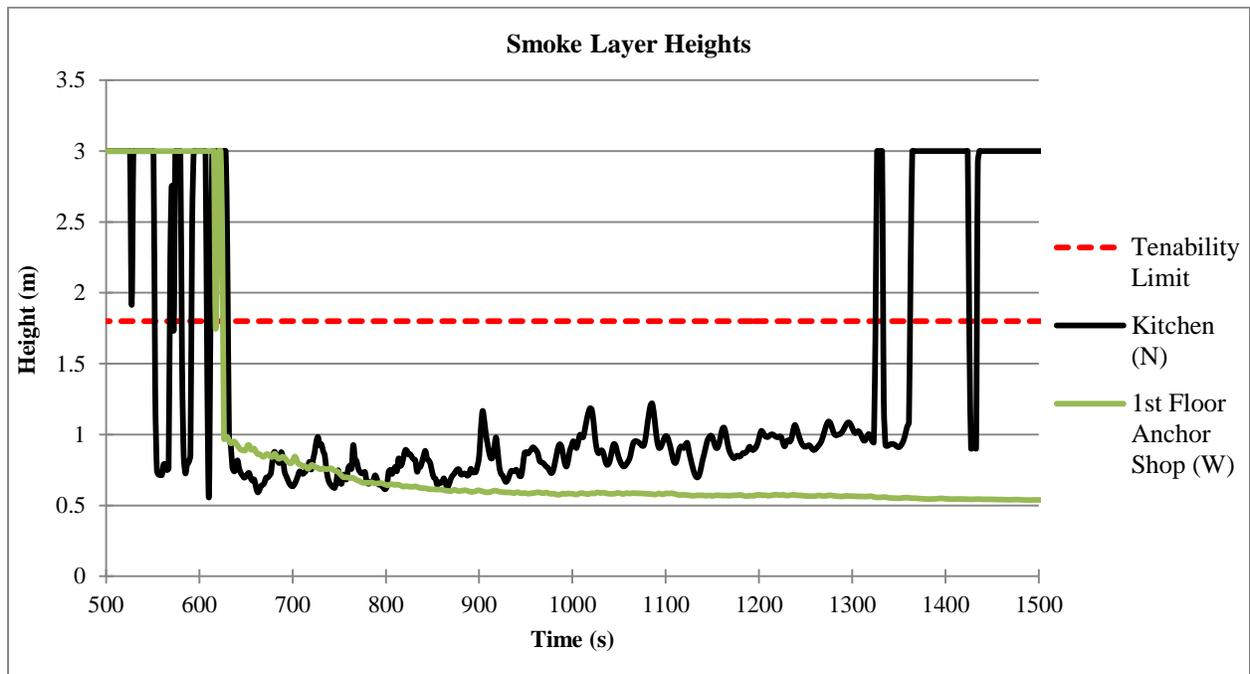
**Figure 77. Time duration when smoke layer exceeds the tenability limit during post-earthquake fire scenario**
