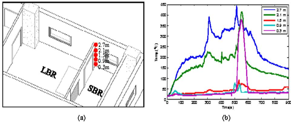
Fig. 11. Locations of thermocouples and temperature profile in LBR-2 fire test
