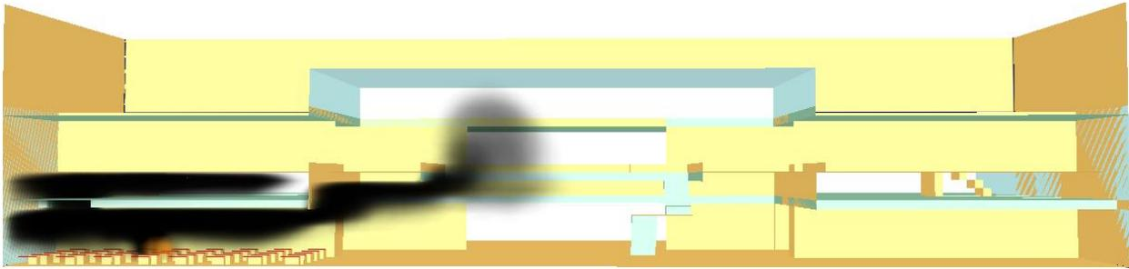
**Figure 74. WPI Mall elevation view in Smokeview in the initial growth stage of the fire**
