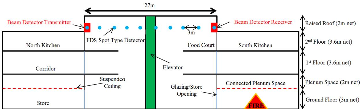
Figure 47. FDS spot type detector location
