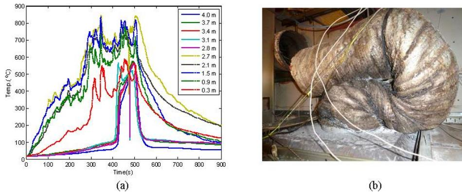
Fig. 5. Temperature increase in the space above LBR ceiling (a) and flexible duct rupture (b)
