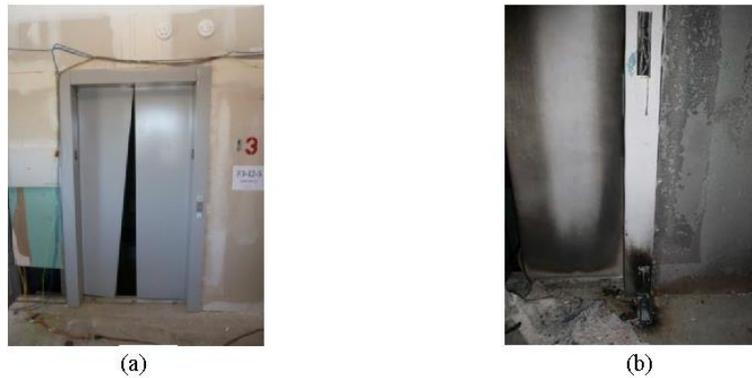
Fig. 4. Damaged elevator door after motion tests (a) and melted elevator button after EL-1 (b)
