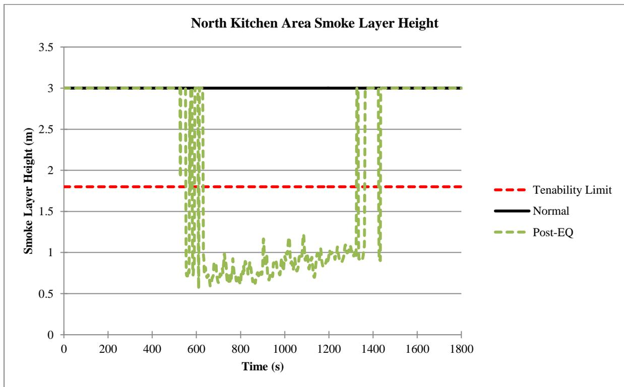
Figure 85. Smoke layer height comparison in North kitchen area
