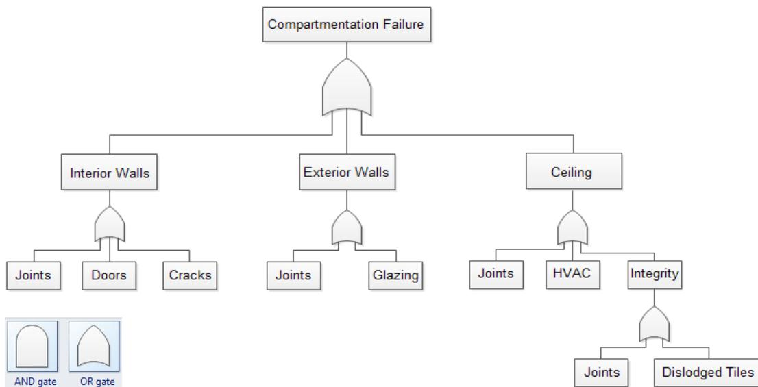
Figure 22. Representative compartment barrier fault tree analysis
