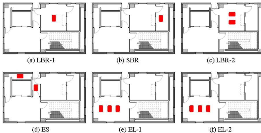
Fig. 3. Fuel locations in each test, a red box representing a heptane pan
