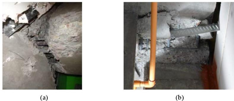
Fig. 8. Structural damage after the motion tests in the second floor: north center column and east beam connection (a) and northwest column and the 3<sup>rd</sup> floor slab connection (b)
