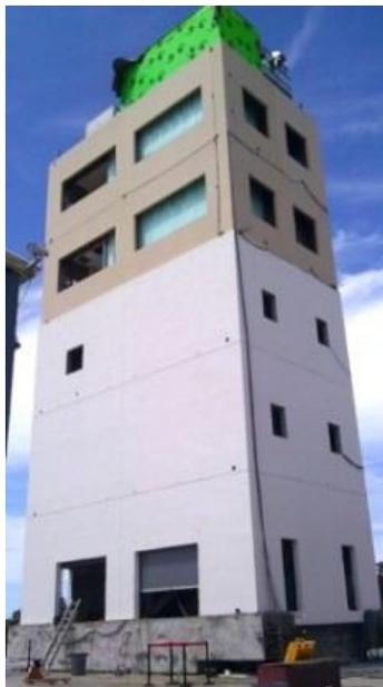
Figure 1. Building specimen built on top of the LHPOST
