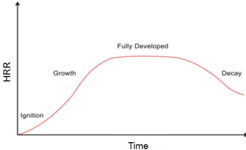
**Figure 16. Generalized fire curve**
