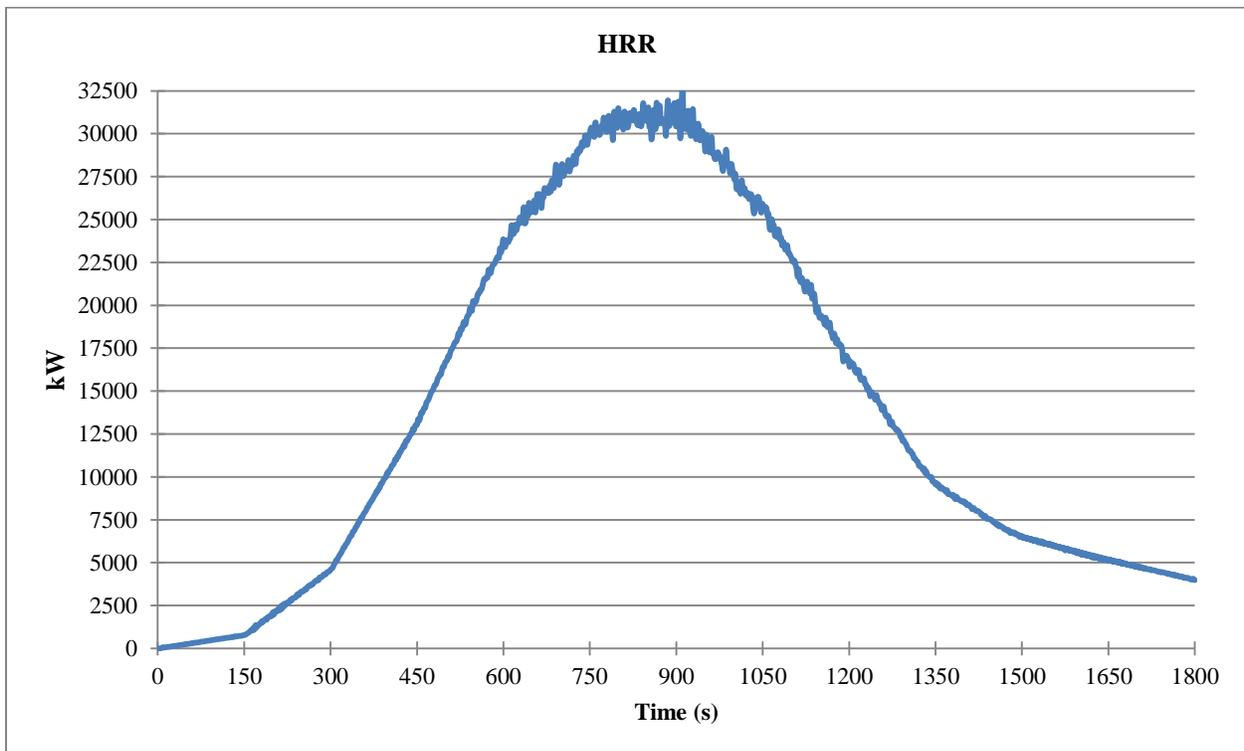
Figure 71. Post-earthquake fire building HRR Curve
