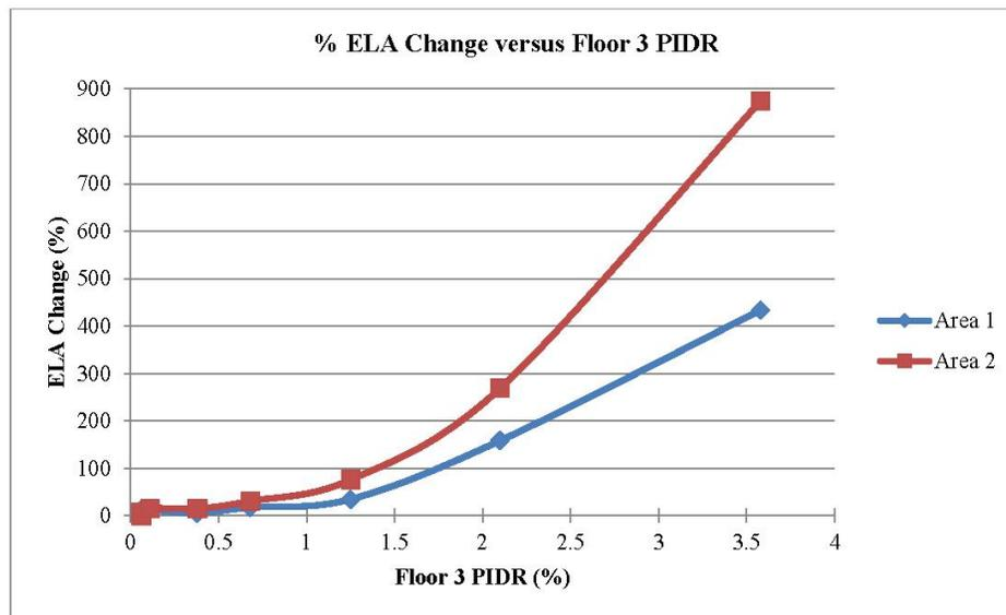
Fig. 15. Plot of % ELA change relative to ‘Before BI-1’ versus PIDR of Floor 3
