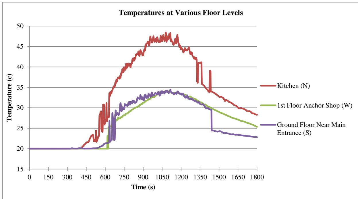
Figure 78. Post-earthquake fire upper layer gas temperatures at various locations
