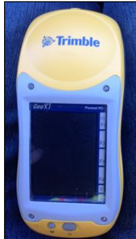
Figure 25 Trimble™ device used for obtaining GPS locations while inventorying
