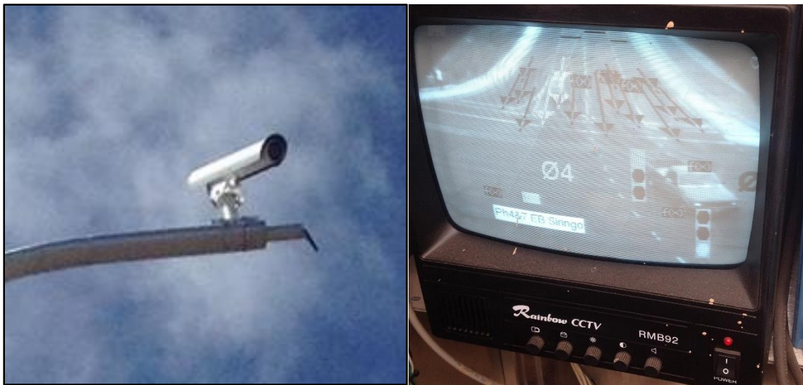
Figure 13. CCTV used for detecting vehicles at intersections to manage traffic light signals (Left). Video camera zones used in traffic signaling detection (Right).
