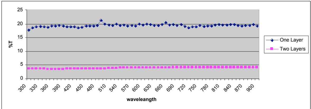
**Figure 6: Graph of %Transmittance vs. Wavelength for one and two layers of desert soil.**
