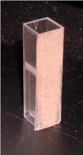
**Figure 5: Cuvette with soil used in spectroscopy procedure**
