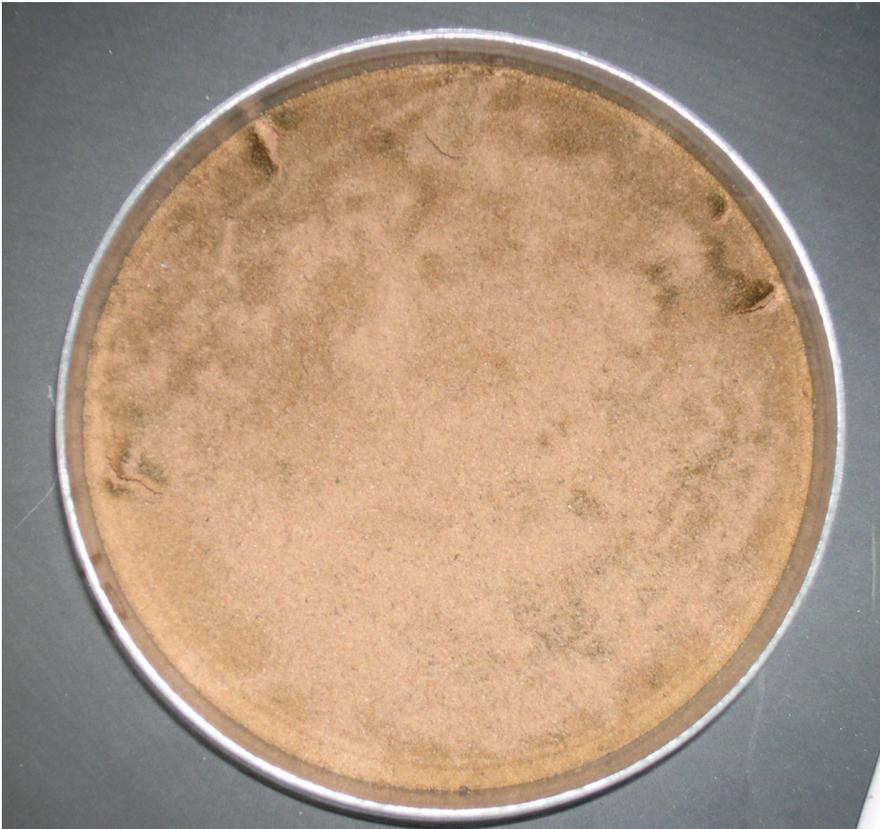
**Figure 7: Soil culture after 12 wet cycles. Note the dark patches and the fractured surface. The surface lift is easily seen in the top picture. The bottom shows variation in soil color as a result of cyanobacterial growth.**
