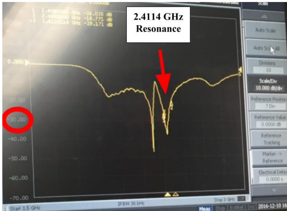
Figure 25. Tuning of Receive Antenna -20 dB Resonance This photo depicts the tuning of the receive antenna of the radar. It demonstrates the resonance behavior at a power level of about -40 dB at a frequency of 2.41 GHz. This resonance was slightly above the expected frequency value of 2.4 GHz, but still demonstrated the behavior that was expected of an antenna operating in the correct frequency band.
