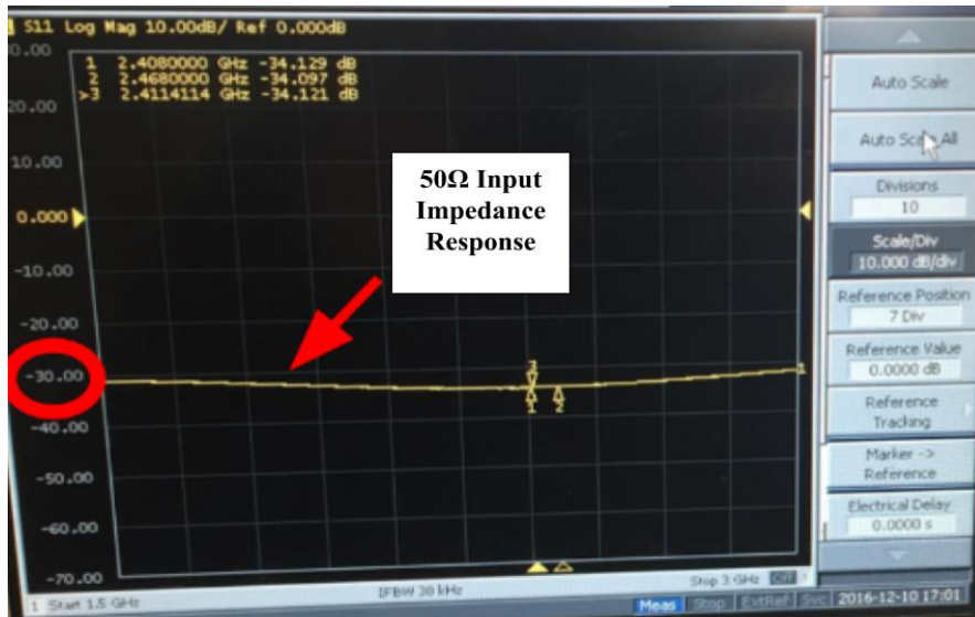
Figure 23. Baseline Calibration Magnitude Response of Spectrum Analyzer with 50 \Omega Input
