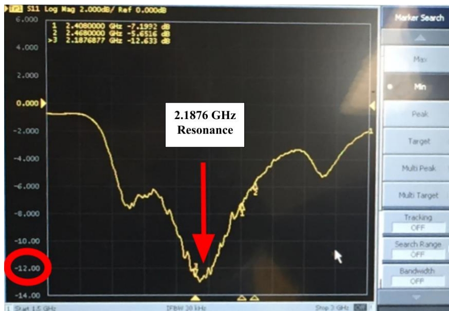
Figure 24. Tuning of Transmit Antenna -12 dB Resonance
