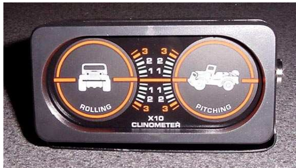
Figure 3- Dash Mounted Inclinometer 7
