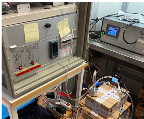
Figure 4.8: Photo of the first test rig with spark discharger machine in the top right, Condensation Particle Counter in the left, and the virtual impactor and flow controller in the bottom right
