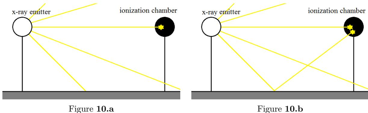
**Figure 10:** Figure 10.a shows the ideal photon emission scenario, where photons (yellow) that are not emitted in the direction of the ionization chamber are not scattered or collected. Figure 10.b shows the effects of scattering. When photons are not absorbed by the environment, they can scatter and enter into the ionization chamber. Because these photons are not originally directed toward the ionization chamber, they alter the expected results.
