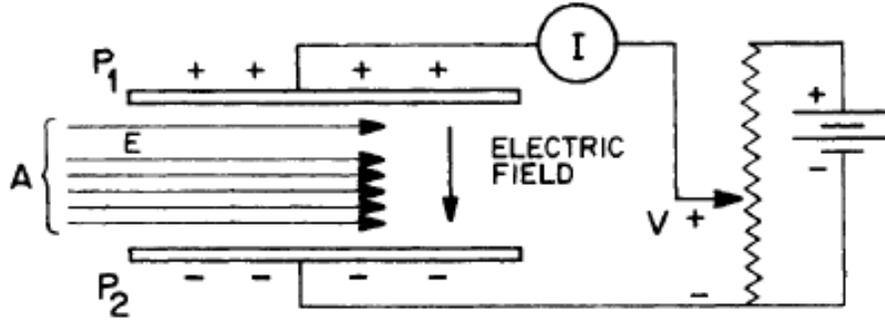
**Figure 9:** An ionization chamber with active area  $A$  is irradiated by a monoenergetic beam of particles that are fully stopped within the chamber. Plates  $P_1$  and  $P_2$  are a cathode and anode, respectively, with a potential difference  $V$  across them. The ion pairs created by the incoming beam create current  $I$  when they collide with the cathode.<sup>7</sup>
