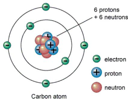
**Figure 1:** The Bohr model of an atom.<sup>1</sup>
