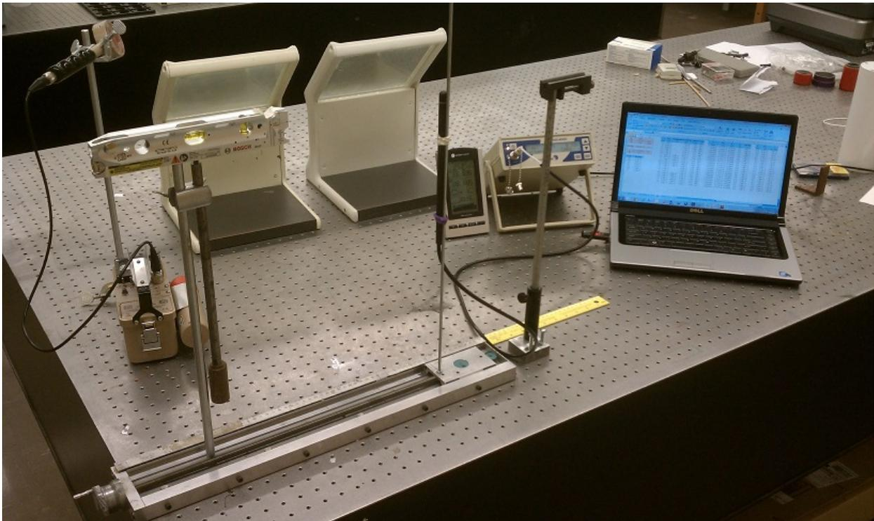
**Figure 13:** A picture of the completed seven-distance apparatus.
