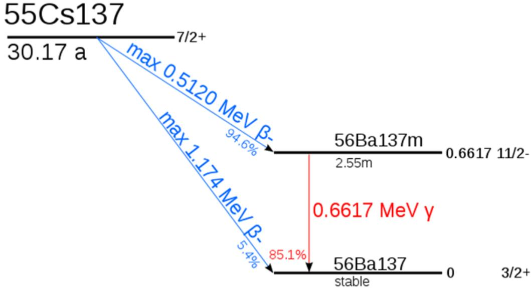
**Figure 5:** The decay scheme of Cs-137.<sup>4</sup>
