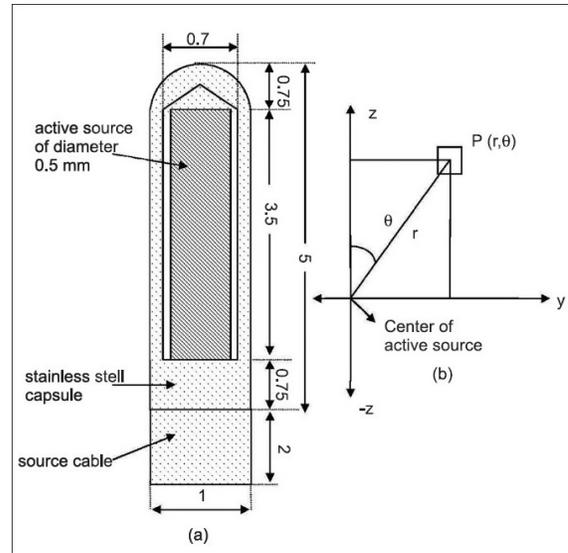
**Figure 7:** Diagram of the components of a brachytherapy seed.<sup>6</sup>
