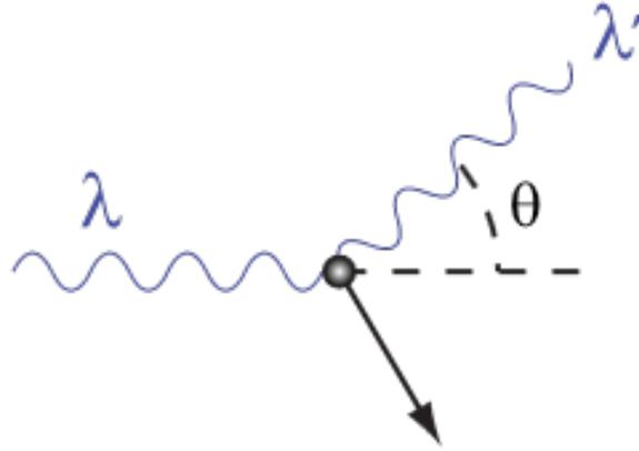
**Figure 4:** A photon with initial wavelength  $\lambda$  interacts with a particle and scatters at an angle  $\theta$  with wavelength  $\lambda'$ .<sup>3</sup>
