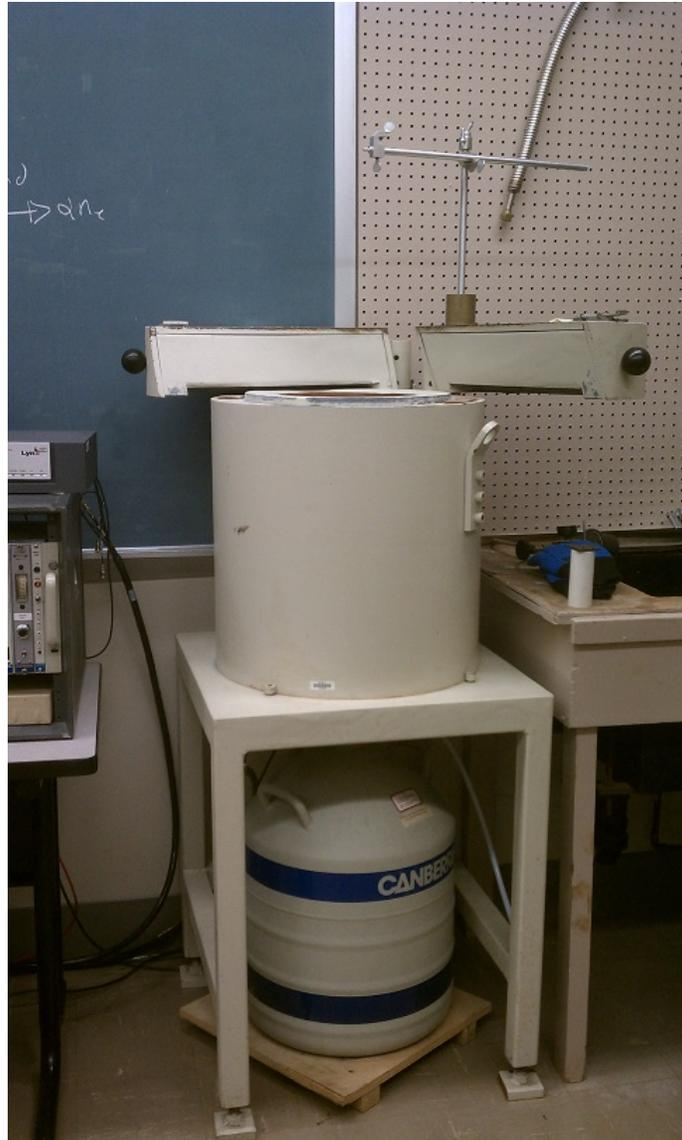
**Figure 14:** A picture of the gamma spectroscopy system used for this project. One can see the lead cylinder that houses the germanium detector sitting on a table above the container of liquid nitrogen to cool the system. The lead doors on the top of the cylinder are swung open, and the source is suspended above the opening on the top of the detector using a pair of metal rods.
