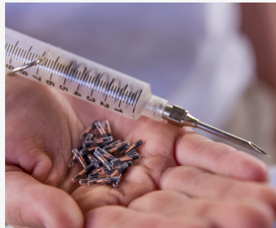
Figure 8 PIT tags before they are injected in the backs of yearling sturgeon
