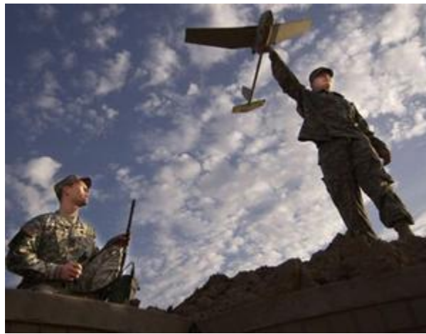
Figure 29 - Launching of RQ-11 Mini-UAV, an UAV that is used for identify possible threats. The UAV acts as second security layer after the first layer of ground sensor [48].
