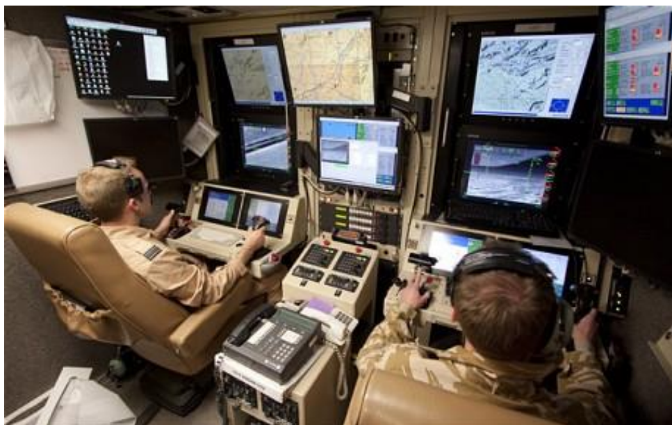
Figure 21 - The UAV command center of a Reaper drone. The pilot is sitting to the left and the sensor operator is sitting on the right. Although the pilot needs to command the plane with the same sense of caution as he would a regular manned aircraft, he is removed from all danger [37].
