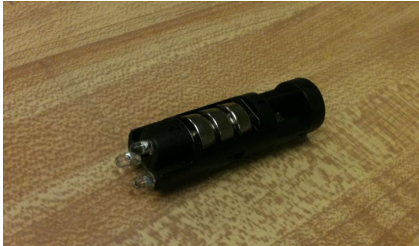
Figure 71 - The LED flashlight that was used had three LEDs with different colors: red, blue and green. The LED had a solid lighting mode as well as a flashing mode.
