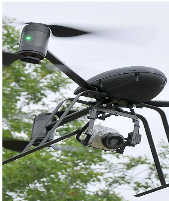
Figure 6 - UAV with thermal Infrared camera to locate people by identifying body heat [11].
