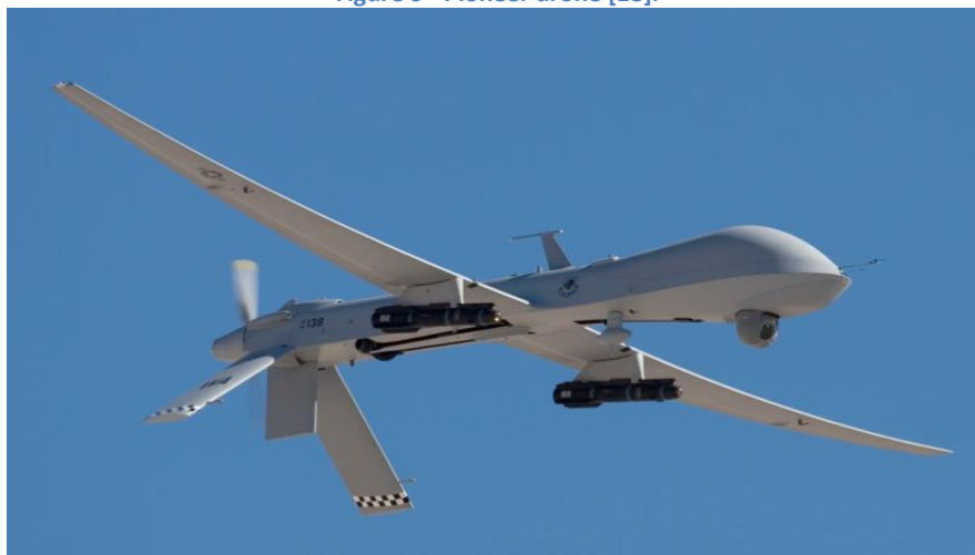
Figure 10 - Predator drone. This and the Pioneer (Figure 7) are two prominent UAVs used by United States defense forces in the recent wars in Iraq and Afghanistan. They have provided invaluable help as they can carry out missions with a dramatically decreased risk for loss of life [19].
