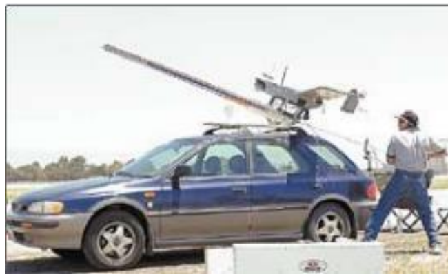
Figure 12 - MLB Bat is prepared to be launched at Moffett Field. The UAVs is launched in flocks like bird and they would gather information for possible risk of wildfire [22].
