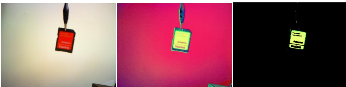
Figure 69 - Color filter process: First image was the original image, second image was converted to HSV color plane and last one was filtering out non-red pixels.
