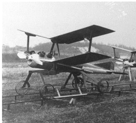
Figure 19 - Kettering Bug by Charles Kettering and Dayton Wright Airplane Company in 1918. The plane has simple autonomous system designed for finding and destroying enemy aircraft [35].
