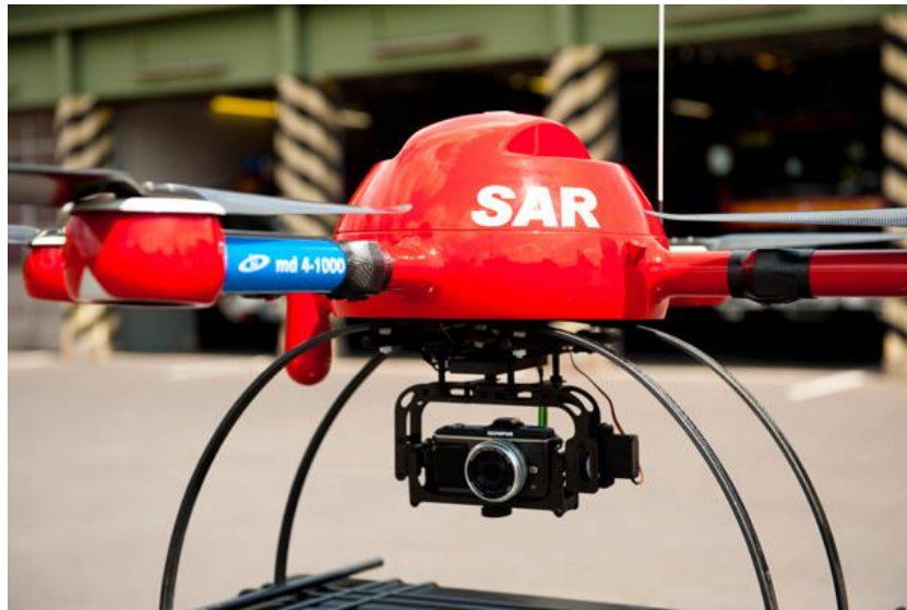
Figure 30 - A search and rescue UAV that is used for finding missing people. The UAV was developed by Flat Eight Productions, Inc. [49].
