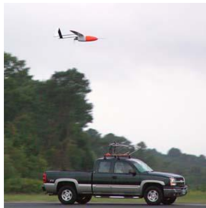
Figure 11 - Aerosonde UAV is being released from its transport vehicle to fly into Tropical Storm Ophelia in 2005. Its mission is to gather weather information for better understanding of tropical storm [21].
