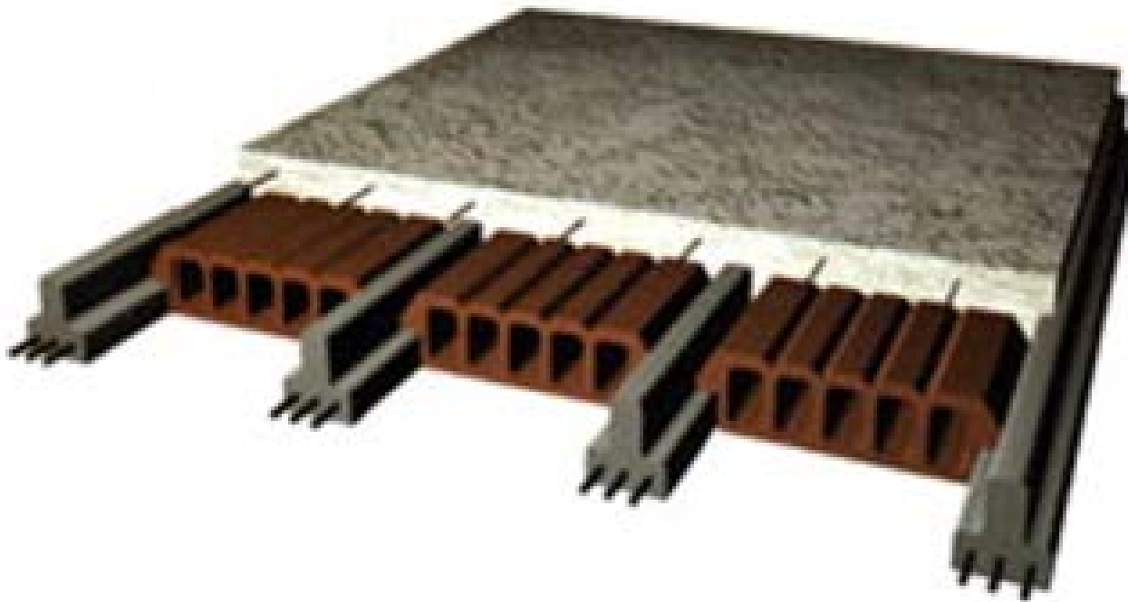
Fig. 2. Geometry of the multilayer one-way slab.
