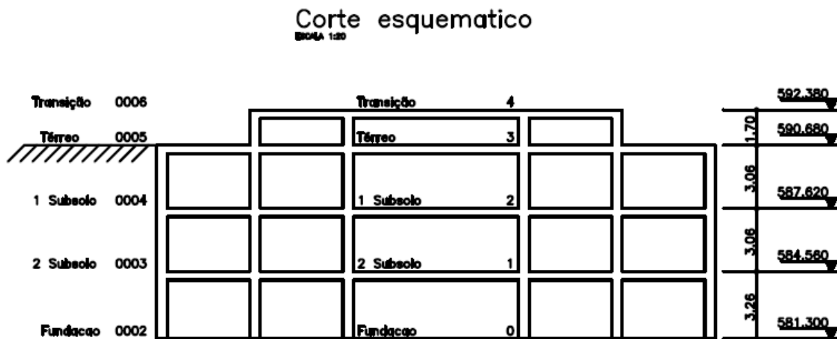
Figure 22 Schematic Section showing Transition and Sub Levels of Structural Masonry to Reinforced Concrete Foundation Structure
