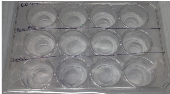
Figure 14: Attachment assay sample preparation. A 12 well plate filled with electrospun material samples placed into the bottom of wells and held in place with PDMS weighting washers.
