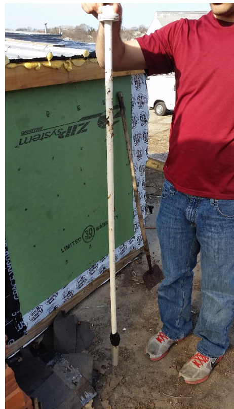
Figure 13: Final thermometer design attached to feed tube cap
