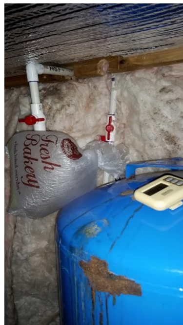
Figure 18: Grocery bag capturing biogas
