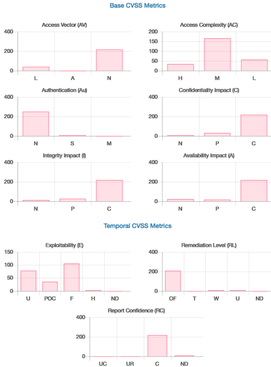
Figure 4.4: Example of VV's graphs displaying the CVSS metrics. Both Base and Temporal CVSS Metrics are extracted from their respective CVSS vector strings in each vulnerability report item from a .nessus scan.
