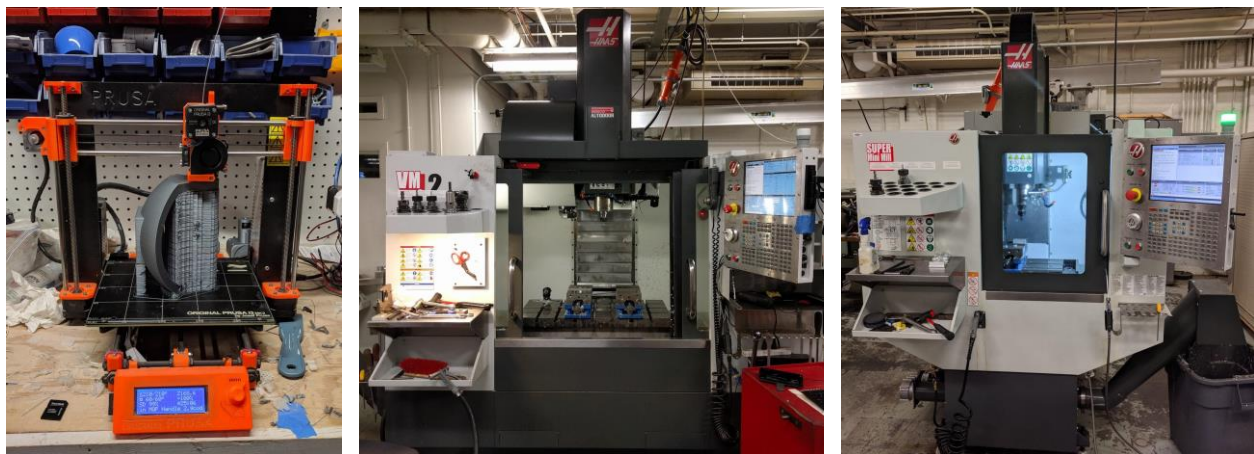
Figure 13.) FDM 3D Printer (Left), Haas VM2 Mill (Center), Haas Super Mini Mill (Right)
