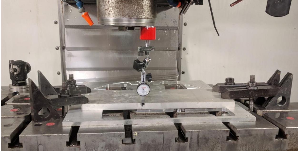
Figure 16.) Toe-clamp Setup with Sacrificial Plate for Waterjet Part
