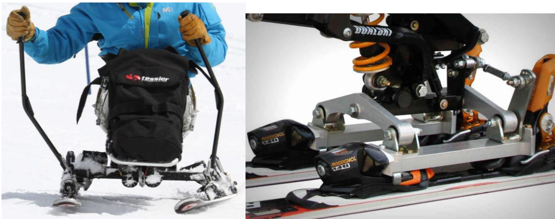
Figure 2: Tessier Snow’Kart (left) and Dualski four-bar mechanism (right)
