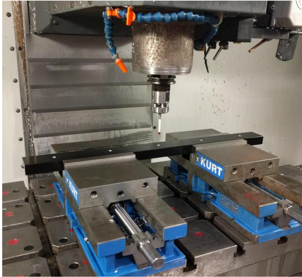
Figure 15.) Setup for Light weighting of 600mm Linear Rail
