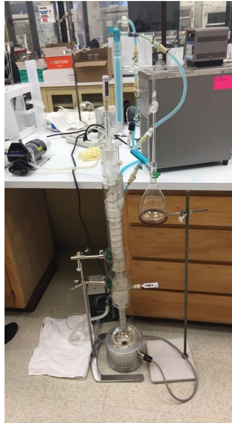
Figure 9: Steam Stripping Column Set-up
