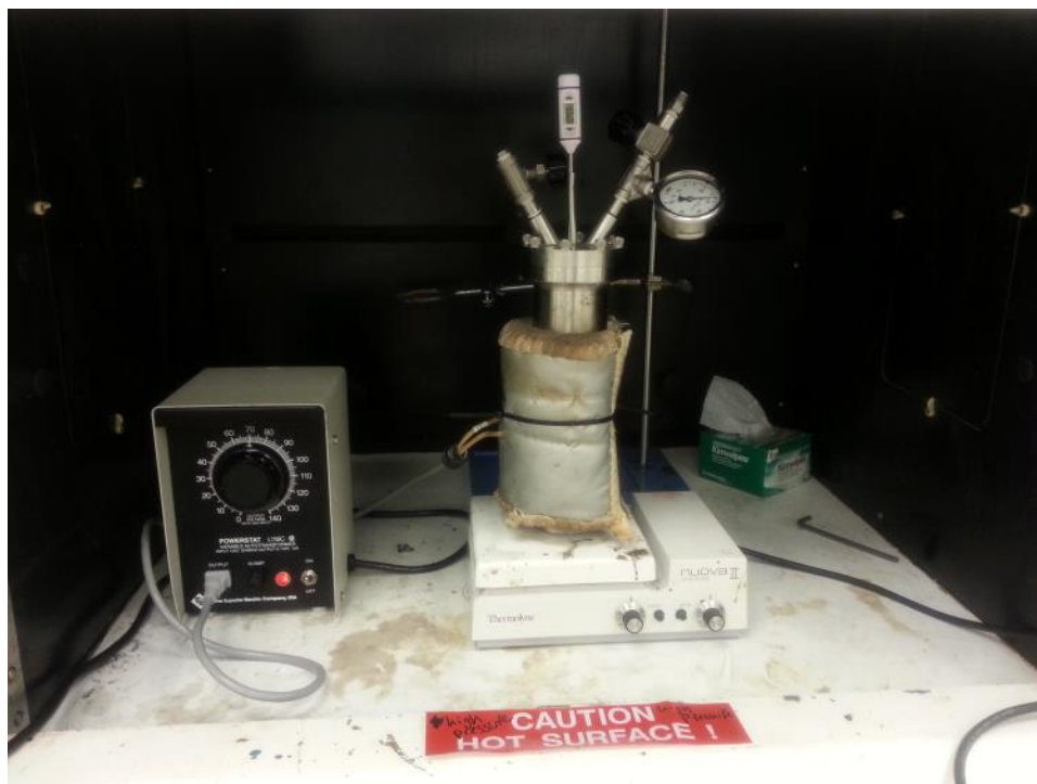
Figure 4: High Pressure Soxhlet Extractor (used for cooking)
